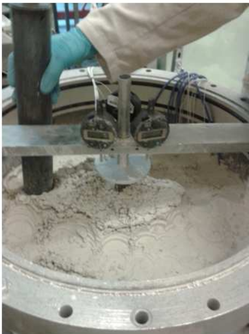
Figure 2.19. First stages of clayey soil compaction
