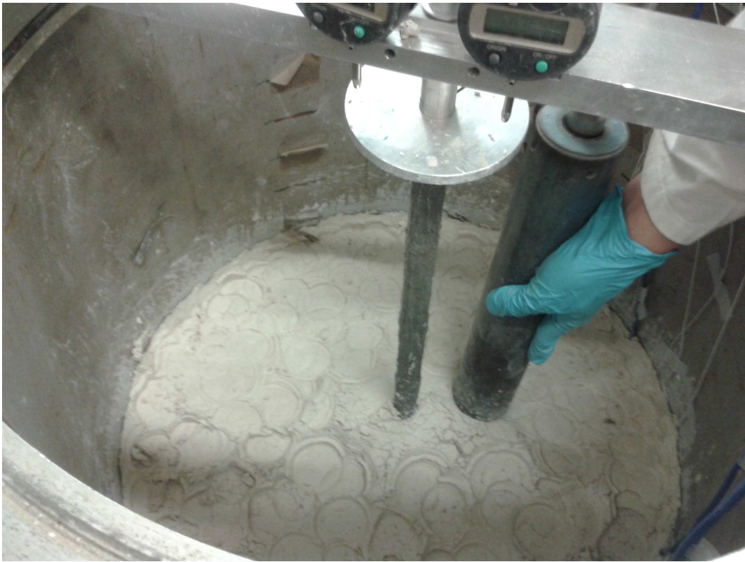
Figure 2.19. First stages of clayey soil compaction
