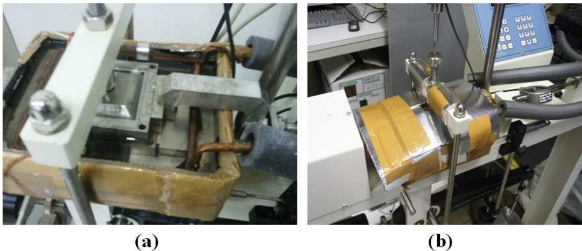
Figure 4.2 (a) View of the shear box with copper tubes and water inside (b) Thermal insulation of the shear box
