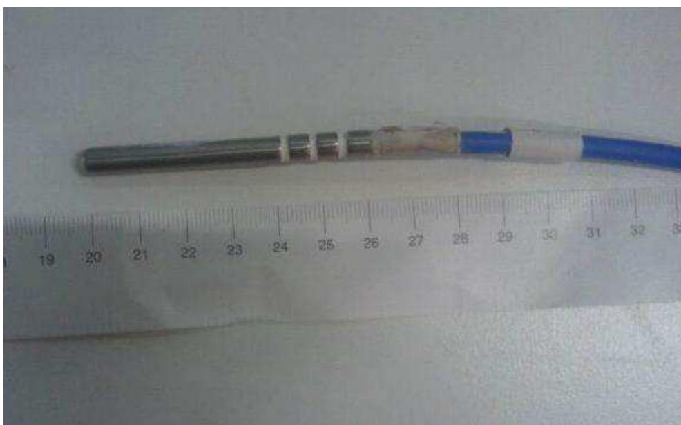
Figure 2.9 Detail on the utilised temperature transducer
