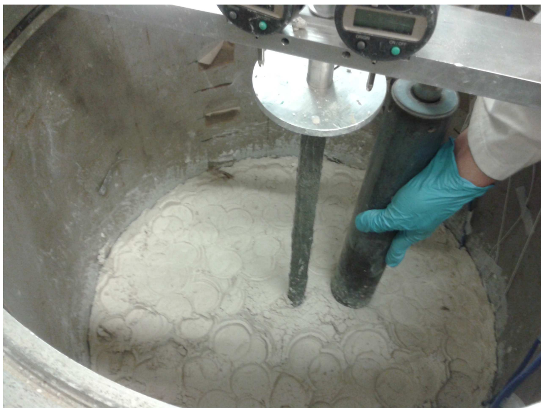
Figure 2.19. First stages of clayey soil compaction
