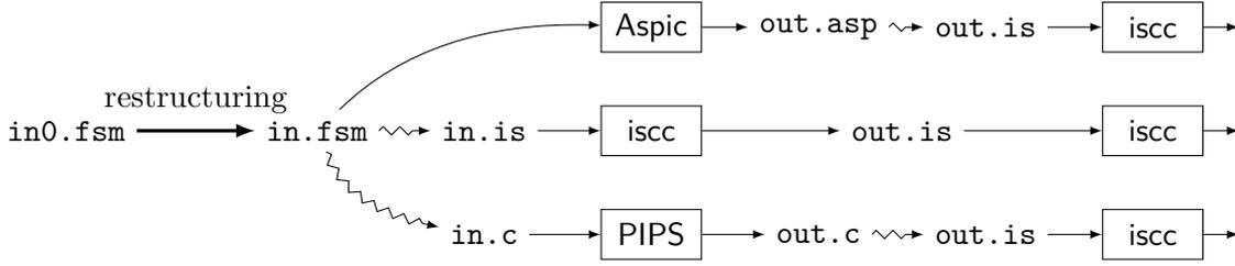
Figure 9.1: Analysis steps within ALICE, using restructuring transformations
