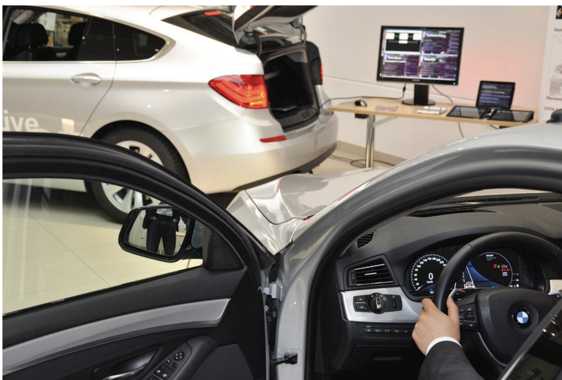
Figure B.9: Active Brake Prototype Demonstrator at Car2Car Forum 2012: The sending vehicle is shown in the background (brake lights engaged). The screen in the background shows details of the key distribution protocol and secure communication: console outputs of brake sensor, key master and brake unit are revealed. In the foreground, the receiving vehicle shows a warning message to the driver: A white vehicle with brake lights appears on the instrument cluster's display.
