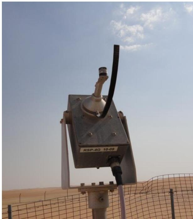
Fig. 4.3: The rotating shadowband radiometer. In this picture the shadowband is still and below the horizon of the photodiode. © Yehia Eissa, 2012.
