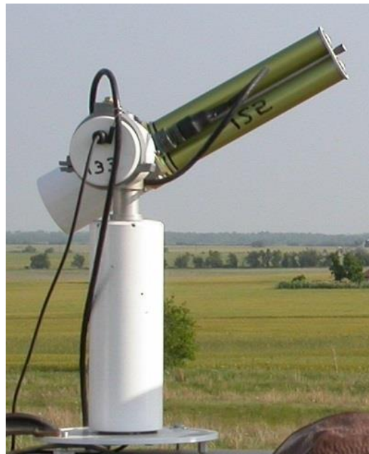
Fig. 4.4: The Cimel 318 Sun photometer used in the AERONET stations (image from: http://www.cimel.fr/?instrument=photometre-multi-bandes-soleilciel ).
