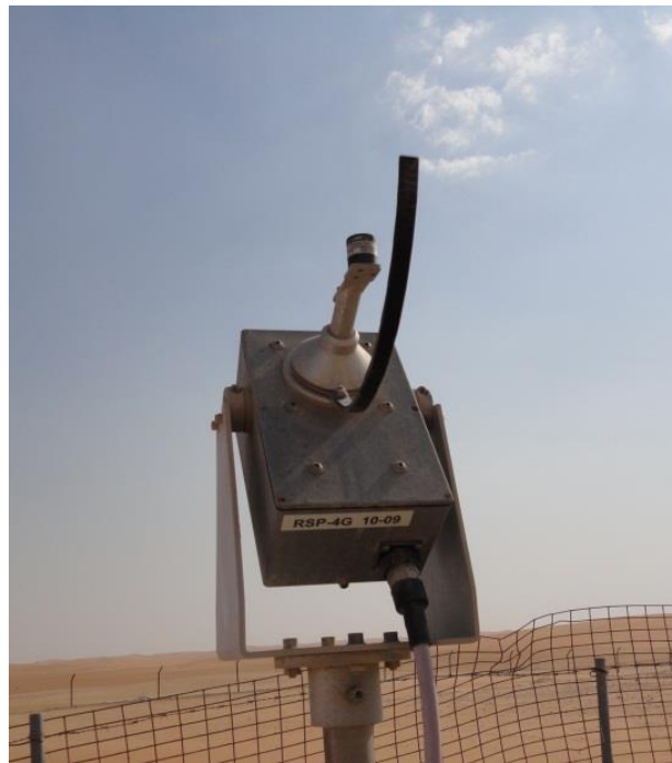
Fig. 4.3: The rotating shadowband irradiometer. In this picture the shadowband is still and below the horizon of the photodiode. © Yehia Eissa, 2012.
