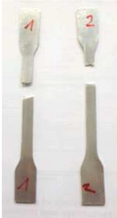
FIGURE E.2 – Eprouvettes de traction.
