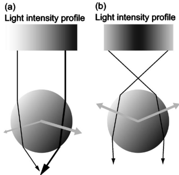
**Figure 3.1: Laser ray geometry within a dielectric bead.** The rays are refracted within the bead. The change of impulse given to the photons is compensated by an equal and opposite impulse on the bead. (a) shows that a lateral movement away from the centre produces a net force towards the centre of the beam. (b) shows a similar reaction to movement of the bead away from the focus of the beam along the beam’s axis. Figure reproduced from [169].
