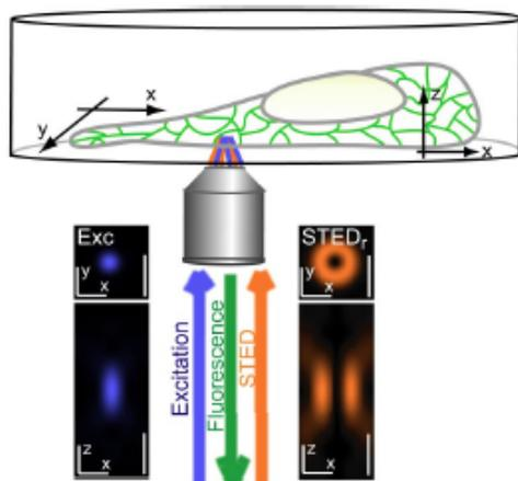
**Figure 1.7: Conceptual image of STED.** An excitation beam is followed by a doughnut shaped stimulated emission beam that serves to reduce the size of the remaining excitation area. Figure reproduced with modifications from [85].
