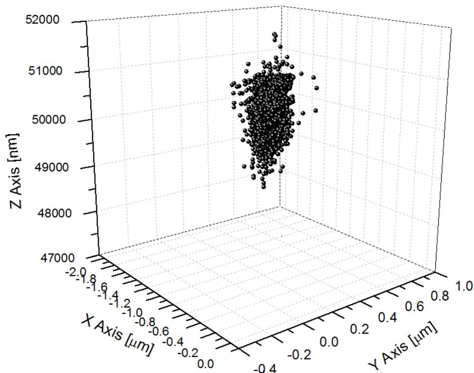
**Figure 6.8: Trajectory of stationary NP showing the mechanical drift of the system.** Trajectory of a NP stuck to a glass surface. Acquisition occurred during a time of 69.1 minutes. The trajectory starts at the 50  $\mu\text{m}$  position and fluctuates due to mechanical drift of the setup within the range of  $49.1 \pm 0.2$  to  $51.4 \pm 0.2$   $\mu\text{m}$ .
