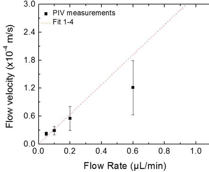
**Figure 4.8: Calibration curve relating injection rate to flow velocity in the microchannel.** This curve represents the relationship between the injection rate of liquid into the channel and the flow speed of the liquid at the position of the NPs observed. The errors are the standard deviation of the 10, 10, 53, and 8 measurements for the flow rates of 0.05, 0.1, 0.2, and 0.6  $\frac{\text{m}}{\text{s}} / \frac{\mu\text{L}}{\text{min}}$ , respectively.
