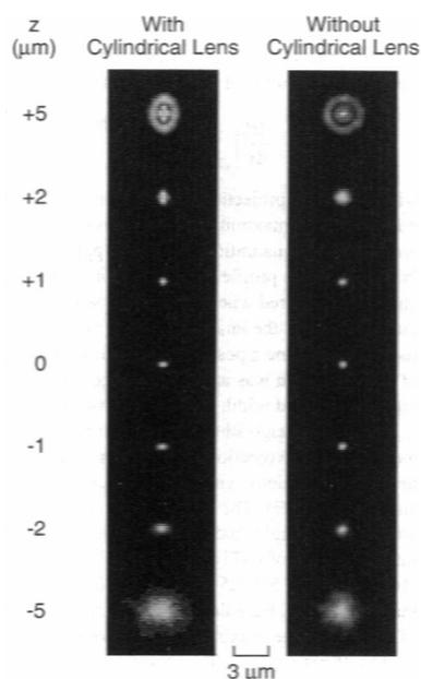
**Figure 6.4: Diagram of the fluorescent signal detected using a cylindrical lens.** Difference in PSF radius and shape as the fluorophore is displaced from the focal plane. Without the addition of a cylindrical lens, the PSF grows in diameter but remains circular. With the cylindrical lens, the shape is modified along with the size. Figure reproduced from [142].
