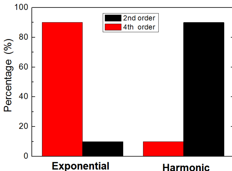
Figure 5.7: Decision-tree results for simulated split trajectories. Using the decision-tree method, the split simulated hopping trajectories are classified into 2nd and 4th order. The trajectories produced using exponential and harmonic potentials were classified by a large majority as fourth- and second-order, respectively. For each case, 50 trajectories were split into 100 individual trajectories, which were then classified. 17 domains of harmonic potentials had to be excluded as not enough data was present in some domains due to a lack of hopping. Using a two-sample t -test with a null-hypothesis that the two distributions have equal means, we can reject the null hypothesis at the 10^{-39}\% significance level.
