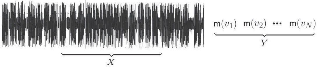
Figure 8.13: Construction of random variables for Horizontal Side-Channel Analysis with a leakage model
