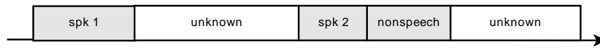
Figure 8.5: Example of an output file provided by ALISP-based audio sequencing and identification.
