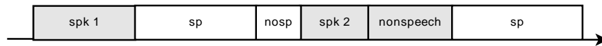
Figure 8.6: Example of an output file provided by the voice activity detection system.
