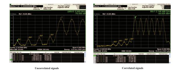
Figure B.4: Measurements at the output of a typical RF Base Station small-signal chain, showing non-linearity products from a six (EDGE) carrier input, indicating it is comparable to 3<sup>rd</sup> order polynomial non-linearity. *Courtesy: NXP Semiconductors, 2011*
