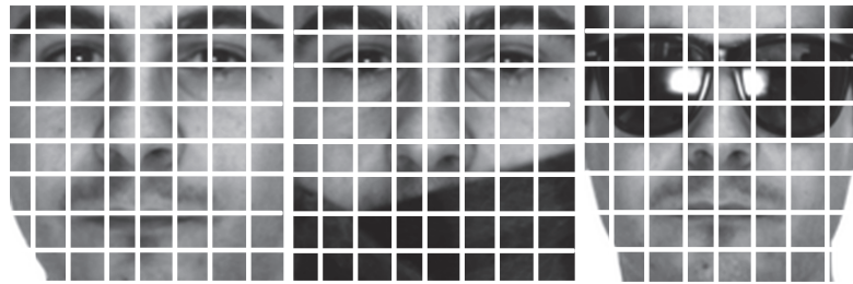
Figure 3.11: The face images are divided into 64 block for LBP based face recognition.
