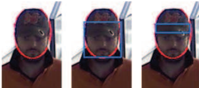
Figure 4.15: Pre-defined ROI 1-3 (from left to right: the whole ellipse, the face region, the upper-eyebrow region).
