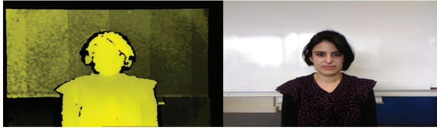
Figure 5.6: Illustration of the RGB-D alignment: the depth map (left) is aligned with the RGB image (right) captured by Kinect at the same time.
