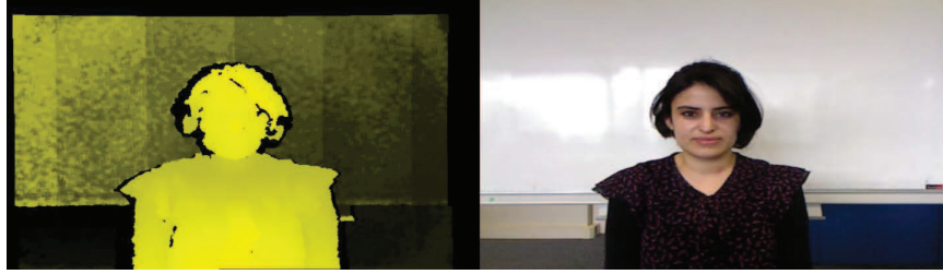
Figure 5.6: Illustration of the RGB-D alignment: the depth map (left) is aligned with the RGB image (right) captured by Kinect at the same time.
