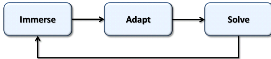
FIGURE 1.1: New computation cycle used to adapt the mesh during the numerical simulation
