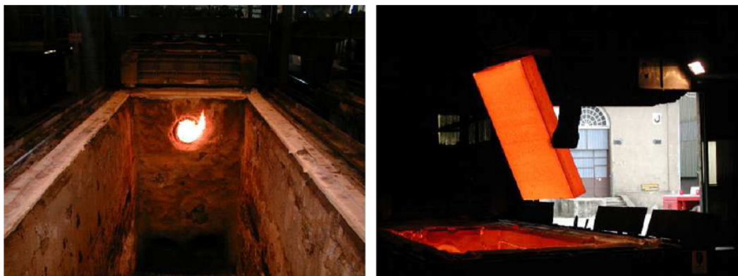
FIGURE 5.9: A top view of the furnace and the immersion of an ingot inside the furnace
