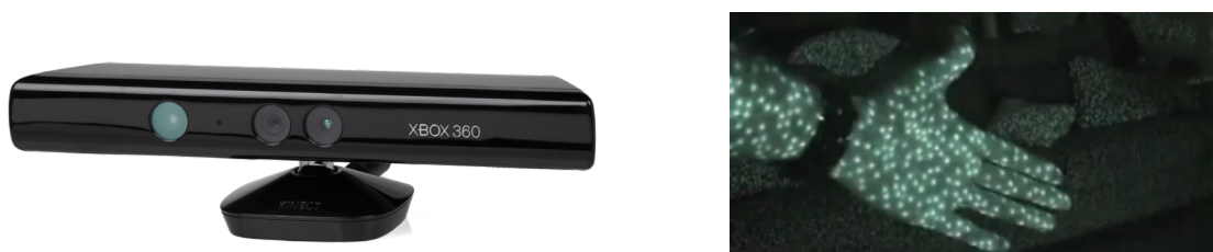
Figure 1.3: Kinect and its structured light patterns.
