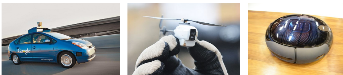
Figure 1.5: Left: Google auto-drive car. Middle: Black Hornet nano air vehicle. Right: Hauzen VC-RE70V SLAM based vacuum robot.
