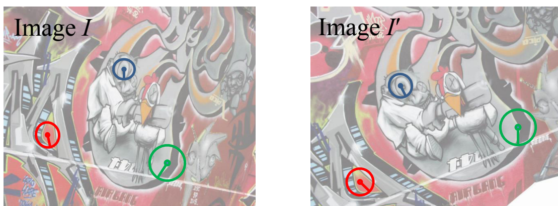
Figure 3.6: Feature detection: specific structures of images are detected, along with a scale (circle radius length) and an orientation (displayed radius).
