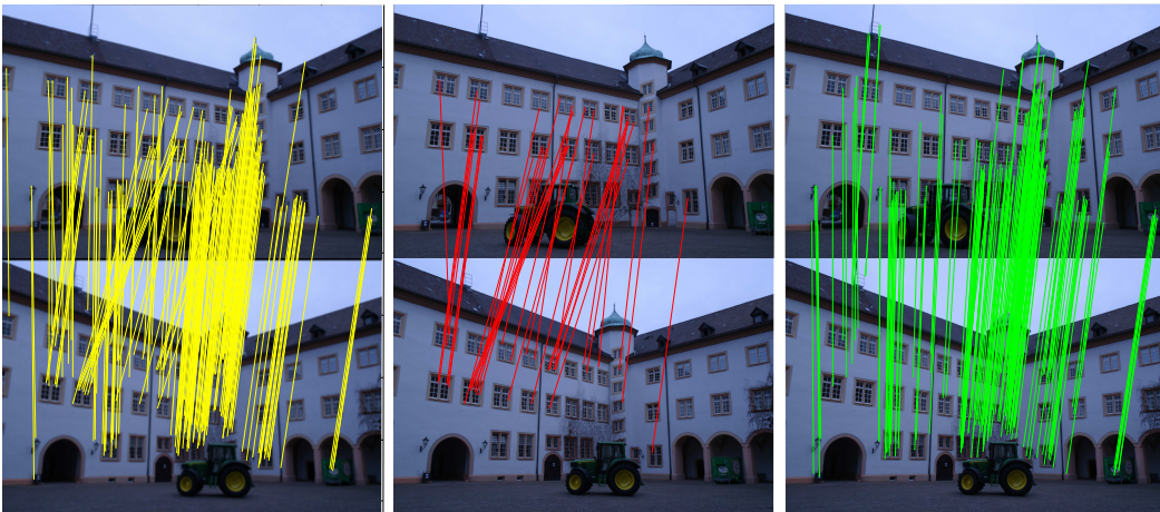
Figure 4.10: Matches on pair of images from Strecha’s Castle-P19 dataset [73]. Left: inliers by ORSA. Middle: false matches near epipolar lines not eliminated by ORSA but rejected by K-VLD. Right: inliers by K-VLD + ORSA. (Symmetric matches; Lowe criterion threshold = 0.8; for readability, only 1/4 matches shown, thus matches may show or hide in different image pairs.)
