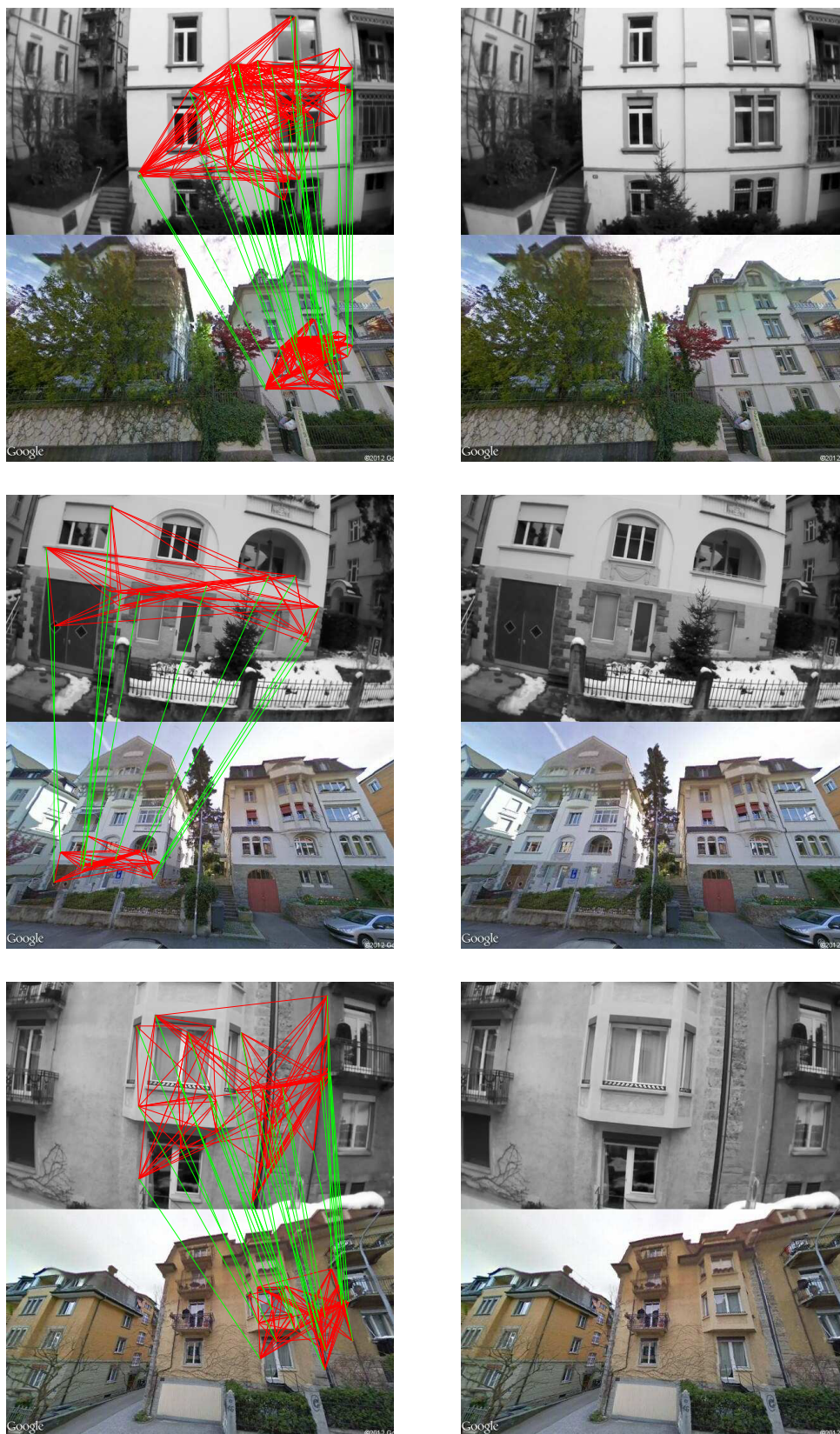
Figure 5.23: Illustration of air-ground matching between images from AR Drone 2.0 and images from Google Street View. Images undergo lens distortion as well as significant viewpoint and scale changes. Left: K-VLD is robust against distortion, and extracts correct matches. gVLD-consistent paths are in red, matches are in green. Right: ORSA fails to find a model within 200,000 iterations in all three cases.
