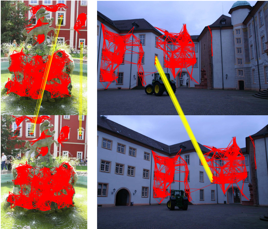
Figure 4.19: Illustration of K-VLD limitation. Outliers are shown in yellow, and validated VLD are in red. Left: First case, where the correct matches of a repetitive group of features are missing. The nearest neighbor principle assigned another set of consistent entities to this group, which is very hard to remove by K-VLD Right: second case, where a subset of features of a repetitive pattern is mismatched, the mismatched cluster of matches overlaps with another cluster of matches.
