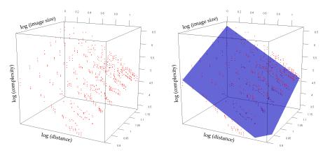
Fig. 16 Experimental space complexities of FDRT graphs in the two pixel-invariance constraints case. The complexities are measured over 676 experiments as a function of image size, varying from  $8 \times 8$  to  $15 \times 15$ , and varying distances between two given constraints limited by the image sizes. Left: 3D log plot of distance, image size and space complexity. Right: least-squares best plane fit (colored in blue).
