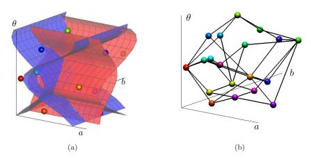
Fig. 3 (a) The parameter space of rigid transformations subdivided by four tipping surfaces, and (b) the associated DRT graph.
