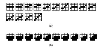
**Fig. 12** (a) The 14 samples of digital lines of length 5, and (b) the half-planes generated by these lines in a 20-neighbourhood.
