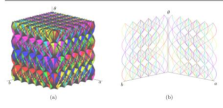
**Fig. 2** (a) Tipping surfaces in the 3D parameter space  $(a, b, \theta)$ , and (b) their cross-sections, namely tipping curves, in the 2D planes  $(a, \theta)$  and  $(b, \theta)$ .
