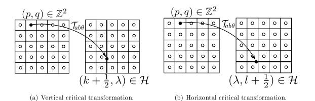
Figure 2.8: Examples of critical transformations  $\mathcal{T}_{ab\theta}$ , each of which moves at least one pixel center onto its boundary which can be either "vertical" (a) or "horizontal" (b). The pixel centers are depicted by dots, while their boundary are depicted by lines.
