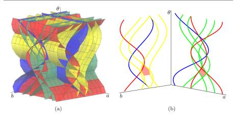
**Fig. 11** (a) Example of tipping surfaces passing through  $\mathcal{R}$  (in red) and not passing through  $\mathcal{R}$  (in blue) in the parameter space  $(a, b, \theta)$ . (b) Its cross-sections  $\mathcal{R}_V$  and  $\mathcal{R}_H$  of (a) on the planes  $(a, \theta)$  and  $(b, \theta)$  respectively.
