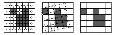
Figure 4.1: Left: binary digital image and the grid modeling its discrete structure. Middle: a rigid transformation applied on this grid. Right: the resulting transformed image, which is not topologically equivalent to the initial image (for instance, the black component is split if it is considered to be 8-connected).
