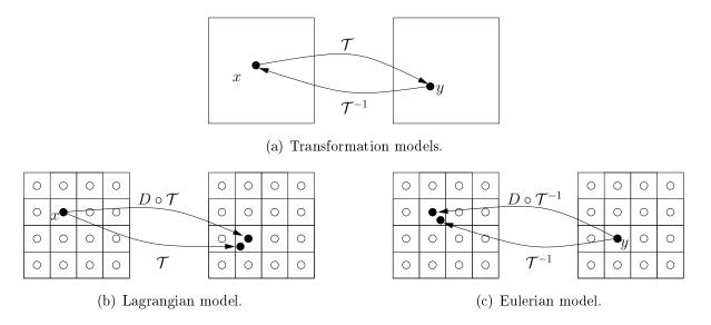
Figure 2.3: Image transformation models: (a) transformation models in  $\mathbb{R}^2$ , (b) Lagrangian and (c) Eulerian transformation models in  $\mathbb{Z}^2$ . (a), (b) and (c) left: image support before transformation; right: image support after transformation. (b) and (c): the digital support  $\mathbb{S} \subset \mathbb{Z}^2$  is depicted by white or black dots, and pixels are depicted by squares.
