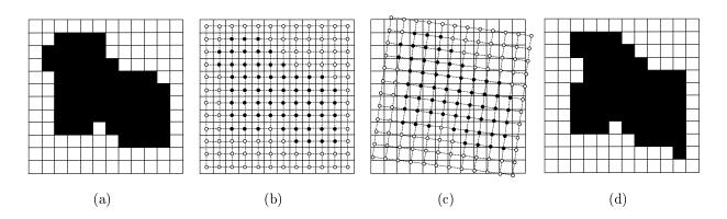
Figure 2.2: Digital rigid transformation. (a) A digital image, (b) the associated grid of the image (a), (c) a rigid transformation applied on the discrete grid of the image (a), and (d) the digital transformed image.
