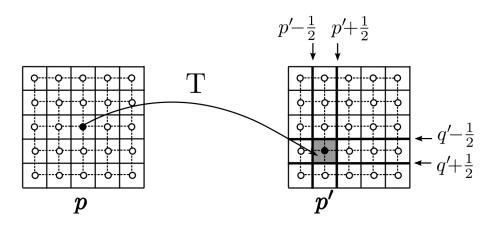
Figure 3.9: A pixel-invariance constraint establishes a correspondence between points  $\boldsymbol{p} = (p, q)$  in the initial space and  $\boldsymbol{p}' = (p', q')$  in the transformed. This leads to a restriction of the authorised rigid transformations in the parameter space.
