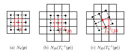
Figure 4.9: Any digital transformation maps a 8-neighborhood into at most a 20-neighborhood. (a) In the transformed space, 8-neighbors of the center point p. (b,c) In the initial space, 20-neighbors of the transformed point of p, for two digital transformations  $T_1$ ,  $T_2$  respectively.
