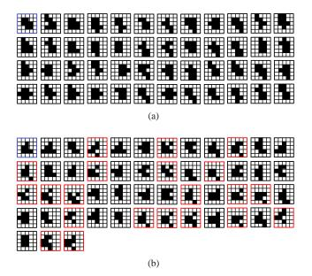
**Fig. 15** (a) A topologically invariant  $5 \times 5$  image (in blue frame), and (some of) its transformations (in black frames). (b) A topologically-variant  $5 \times 5$  image (in blue frame), and (some of) its simple-equivalent (in black frames) and non-simple-equivalent transformations (in red frames).
