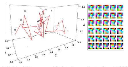
**Fig. 17.** A discrete transition path of the DRT graph in the parameter space  $(a, b, \theta)$  (left) and a sequence of transformed images (right). Each vertex of the path represents a DRT which gives a digital transformed image. The first image corresponds to the identity transformation and the images from left to right and from top to bottom correspond to the vertices ordered in the path.
