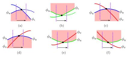
Fig. 13 Classification of simple boundary event points. An event point generated by two tipping curves  $\phi_u$  and  $\phi_v$ : (a,b) changes the boundary from  $\phi_u$  to  $\phi_v$ , (c,d)  $\phi_v$  goes in and out by crossing the upper boundary  $\phi_u$ , and (e,f)  $\phi_v$  goes in and out by crossing the lower boundary  $\phi_u$ .
