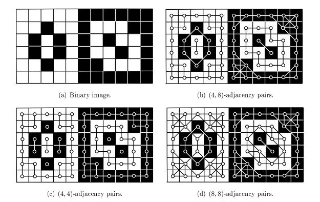
Figure 4.3: (a) A binary image. (b-d) Adjacency graphs of the black and white points in (a), in which we use 4- and 8-adjacencies (b), 4- and 4-adjacencies (c) and 8- and 8-adjacencies (d) for black and white points respectively.
