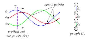
**Fig. 6** Example of a cut  $\gamma$  and its associated graph  $G_{\gamma}$ .
