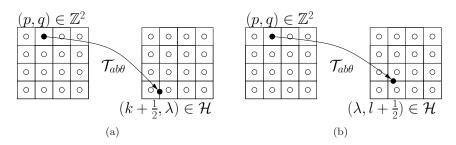
Fig. 1 Examples of critical transformations  $\mathcal{T}_{ab\theta}$ , each of which maps at least one integercoordinate point onto a "vertical" (a) or "horizontal" (b) half-grid point. The integercoordinate points in  $\mathbb{Z}^2$  are depicted by dots, while the half-grid points are depicted by lines.
