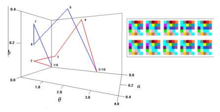
**Fig. 18.** Illustration of two different discrete transition paths with the same starting and ending vertices in a DRT graph: the two paths (left) and their sequences of images (right). The first row images correspond to the red path and the bottom ones correspond to the blue path. (For interpretation of the references to colour in this figure legend, the reader is referred to the web version of this article.)
