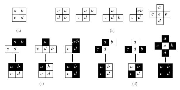
Figure 4.7: (a) A  $2 \times 2$  pixel sample with values a, b, c, d. (b) All the local pixel configurations (up to rotations and symmetries) leading to the sample in (a) when applying digital rigid transformations. (c) Examples of transformations in which the samples preserve the topology of local pixel configurations. (d) Examples of transformations in which the samples are topologically altered.
