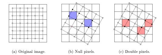
Figure 2.4: Digital rigid transformation is not necessarily bijective. (a) Original image with the associated grid. (b,c) Rigid transformation applied on the grid defined in (a). (b) The blue pixels, containing no images of any discrete points after a digital rigid transformation T (namely, null pixels) show the non surjectivity of T. (c) The red pixels, containing two images of two discrete points after T (namely, double pixels) show the non injectivity of T.
