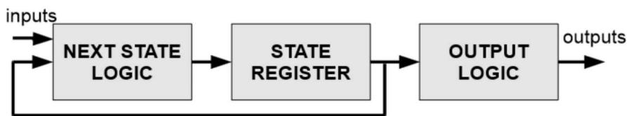
Figure 1.2: Block diagram of a digital circuit including its sequential and combinational parts.
