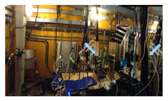
Figure B.3: Full experiment setup showing the FPGA boards, the neutron source and the webcam.
