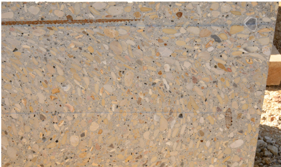
Figure 5.17: On this image we saw how the right border influence the distribution of the aggregates compared to the part on the left under the horizontal (metallic) structure where we can see some preferred orientation of the aggregates.
