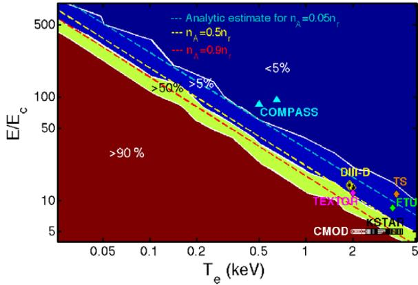
**Figure 8.** The fraction of runaways originating from knock-on collisions ( $n_A/n_r$ ) as modelled in LUKE. The analytic estimate of when 5% (cyan line), 50% (yellow line) and 90% (red line) of the runaways come from avalanche is obtained from equation (23). Non-disruptive scenarios where runaway electrons were generated in several tokamaks are taken from [13] except for the Tore Supra (TS) point (discharge #40719) and COMPASS points (discharge #8555 and #8630).
