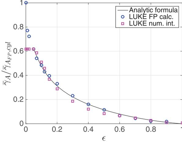
**Figure 7.** Radial dependence of the avalanche multiplication factor from bounce-averaged LUKE calculations (circles), normalized to the avalanche multiplication factor for the cylindrical case  $\epsilon = 0$ . The numerical integration over the knock-on source term in equation (4) with the toroidal dependence in the momentum integration boundary is plotted in squares. The solid line shows the analytic estimate of the growth rate off the magnetic axis from equation (A.4).
