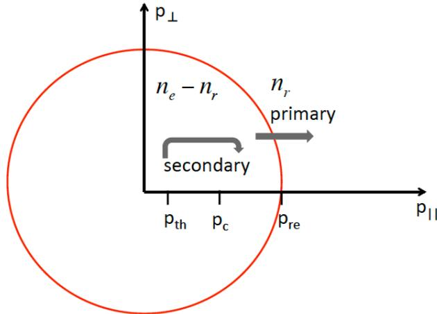
Figure 5.2: The LUKE momentum space is divided into two separate populations: the bulk electrons with momentum  $p < p_{re}$  and the runaway electrons  $p > p_{re}$ . The knock-on collisions between the populations  $n_r$  and  $n_e$  can lead to secondary runaway electrons. Electrons that escape the domain  $p < p_{re}$  either by electrons diffusing through  $p_{re}$  or by getting contribute to the runaway electron population  $n_r$ .
