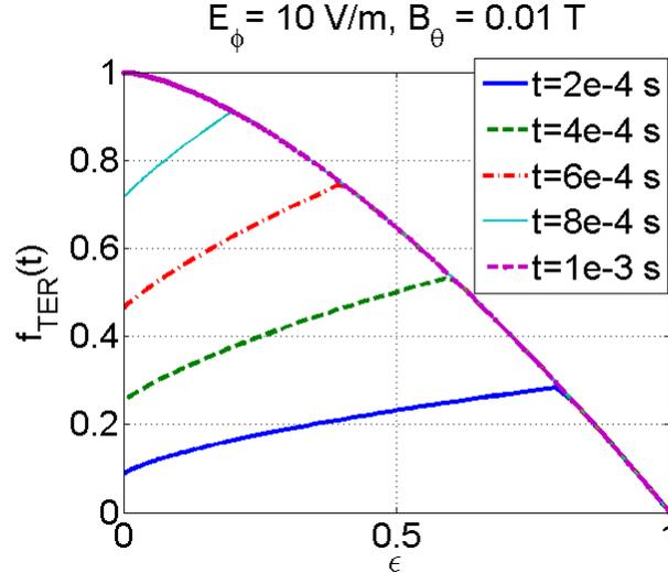
Figure 6.11: The radial distribution function of the trapped-electron runaways, given the initial trapped electron distribution function  $f_T \approx \sqrt{\epsilon}$  for the parameters  $E_\phi = 10$  V/m,  $B_\theta = 0.01$  T and  $R = 1$  m.
