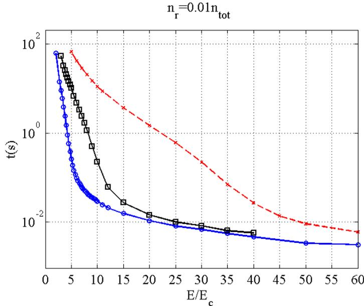
Figure 5.10: The time required for 1% of the initially Maxwellian electrons to run away, for the electron temperature  $T_e = 0.5$  keV (dashed line), 2 keV (solid line and squares) and 5 keV (solid line and circles) .
