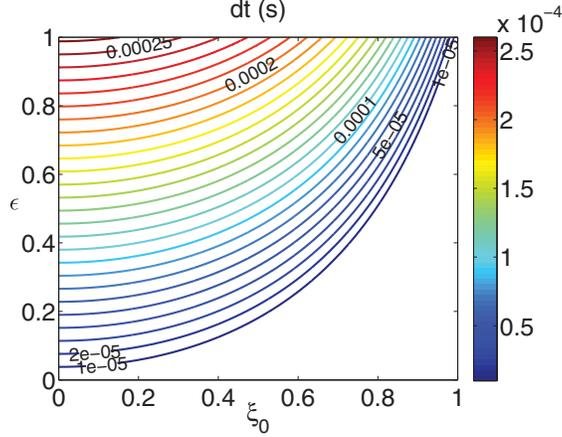
FIGURE 5. Time (s) for trapped electrons at  $(\xi_0, \epsilon)$  to reach the radial position where they become passing electrons, for  $B_\theta = 0.01$  T,  $E_\phi = 38$  V m $^{-1}$  and  $R = 1$  m.
