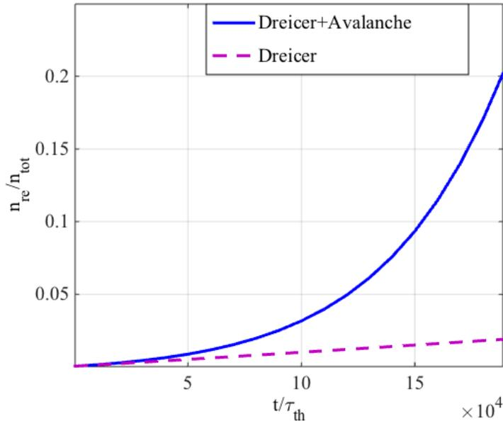
Figure 5.3: The fraction of runaway electrons ( $E/E_c = 30$  and  $T_e = 0.5$  keV) as a function of time normalized to thermal collision time, with and without the avalanche effect due to the knock-on collisions. .
