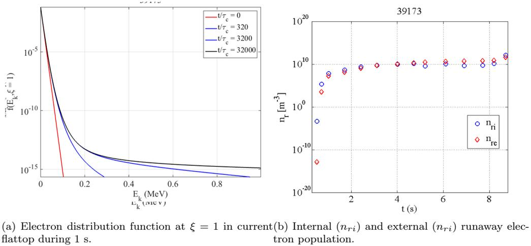
(a) Electron distribution function at  $\xi = 1$  in current flat top during 1 s. (b) Internal ( $n_{ri}$ ) and external ( $n_{re}$ ) runaway electron population.
