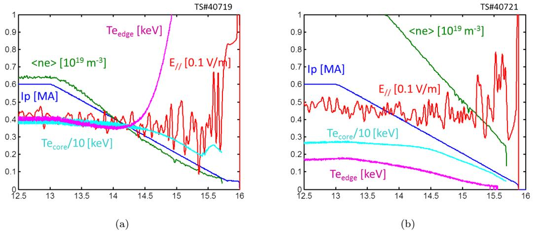
Figure 5.11: Signature of suprathermal electrons on the edge ECE chord at around  $t = 14.5$  s are seen in the Tore Supra discharge #40719 (a). When the density is higher (#40721) (b), there is no sign of supra thermal electrons.
