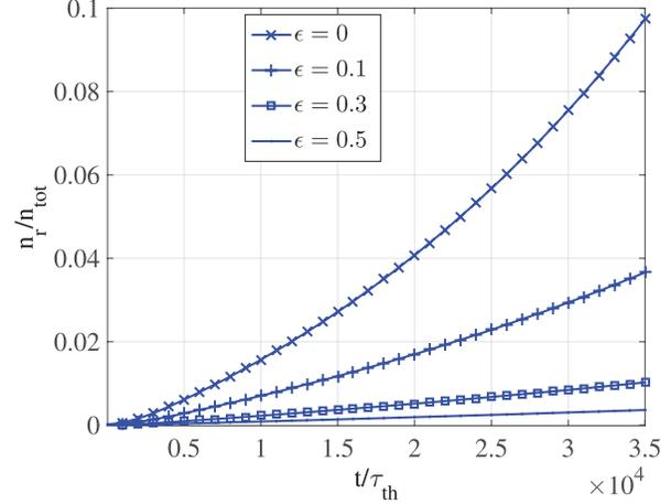
**Figure 5.** The evolution of the runaway electron population, including the avalanche effect owing to knock-on collisions, depends strongly on the radial position in a non-uniform magnetic field configuration, where  $\epsilon = r/R$  is the inverse aspect ratio coordinate.  $E/E_c = 40$ ,  $T_e = 0.5$  keV,  $n_e = 2 \cdot 10^{19} \text{ m}^{-3}$  and the time  $t$  is normalized to the thermal collision time  $\tau_{th} \approx 3.5 \cdot 10^{-6} \text{ s}$ .
