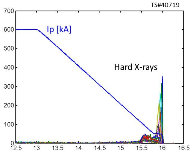
Figure 5.15: HXR data from the vertical camera (channels 1-21) in the energy range  $E_{HXR} = 20 - 200$  keV. The HXR emission produced in the current ramp down in #40719 is a signature of suprathermal electrons, whereas in the higher density discharge #40721 no HXR emission is detected.
