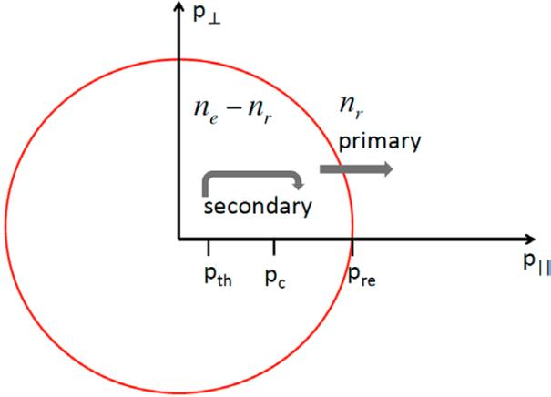
**Figure 1.** The LUKÉ momentum space is divided into two separate populations: the bulk electrons with momentum  $p < p_{re}$  and the runaway electrons  $p > p_{re}$ . The knock-on collisions between the populations  $n_r$  and  $n_e$  can lead to secondary runaway electrons. Electrons that escape the domain  $p < p_{re}$  by diffusion through  $p_{re}$  contribute to the runaway electron population  $n_r$ .
