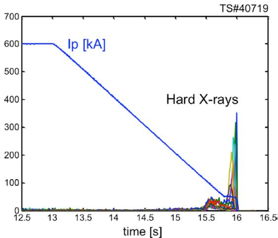
**Figure 11.** HXR data from the vertical camera (channels 1–21) in the energy range  $E_{HXR} = 20\text{--}200$  keV. The HXR emission produced in the current ramp down in 40719 is a signature of suprathermal electrons, whereas in the higher density discharge 40721 no HXR emission is detected.
