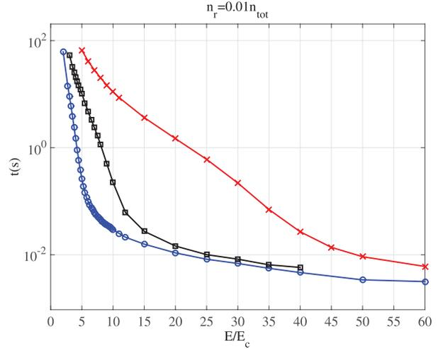
**Figure 9.** The time required for 1% of the Maxwellian electrons to run away, for the electron temperature  $T_e = 0.5$  keV (dashed line),  $2$  keV (solid line and squares) and  $5$  keV (solid line and circles).
