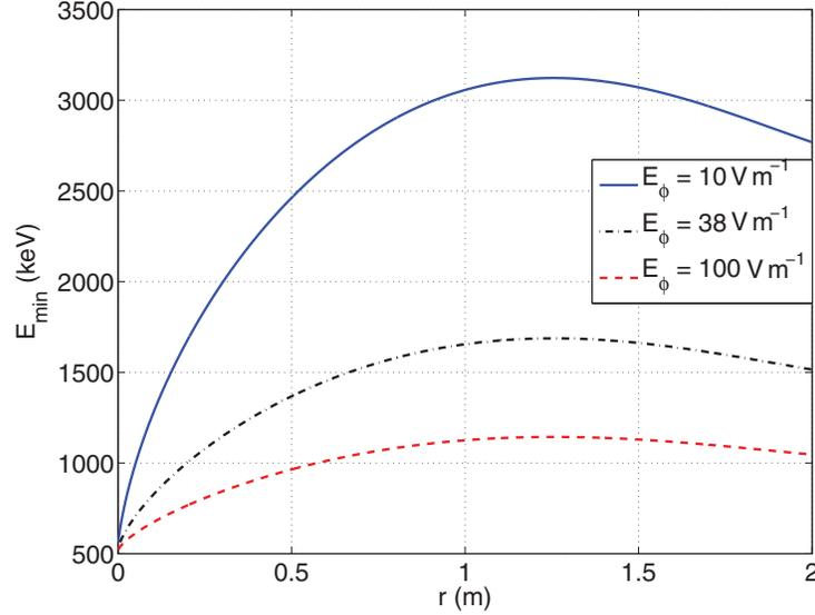
FIGURE 6. The minimum energy needed for the Ware pinch to be faster than the collision time, for the parameters  $E_\phi = 10 \text{ Vm}^{-1}$ ,  $38 \text{ Vm}^{-1}$  and  $100 \text{ Vm}^{-1}$ ,  $n_e = 10^{20} \text{ m}^{-3}$  and  $R = 6.2 \text{ m}$ . The poloidal magnetic field is calculated from a current density profile with a total plasma current of  $I_p = 15 \text{ MA}$ .
