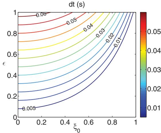
FIGURE 4. Time (s) for trapped electrons at  $(\xi_0, \epsilon)$  to reach the radial position where they become passing electrons, for  $B_\theta = 0.05$  T,  $E_\phi = 0.8$  Vm $^{-1}$  and  $R = 1$  m.
