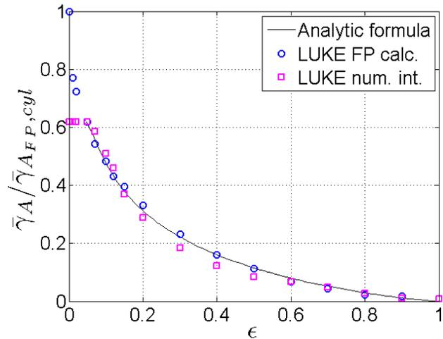
Figure 6.3: Radial dependence of the avalanche multiplication factor from bounce-averaged LUKE calculations (circles), normalized to the avalanche multiplication factor for the cylindrical case  $\epsilon = 0$ . The numerical integration over the knock-on source term in Eq. 4.28 with the toroidal dependence in the momentum integration boundary is plotted in squares. The solid line shows the analytic estimate of the growth rate off the magnetic axis from Eq. 6.27.
