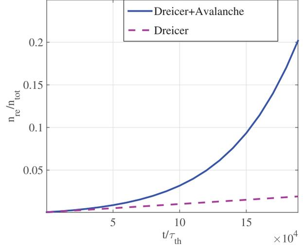
**Figure 2.** The fraction of runaway electrons ( $E/E_c = 30$ ,  $T_e = 0.5$  keV and  $n_{tot} = 2 \cdot 10^{19} \text{ m}^{-3}$ ) as a function of time normalized to thermal collision time (here  $\tau_{th} \approx 3.5 \cdot 10^{-6}$  s), with and without the avalanche effect due to the knock-on collisions.
