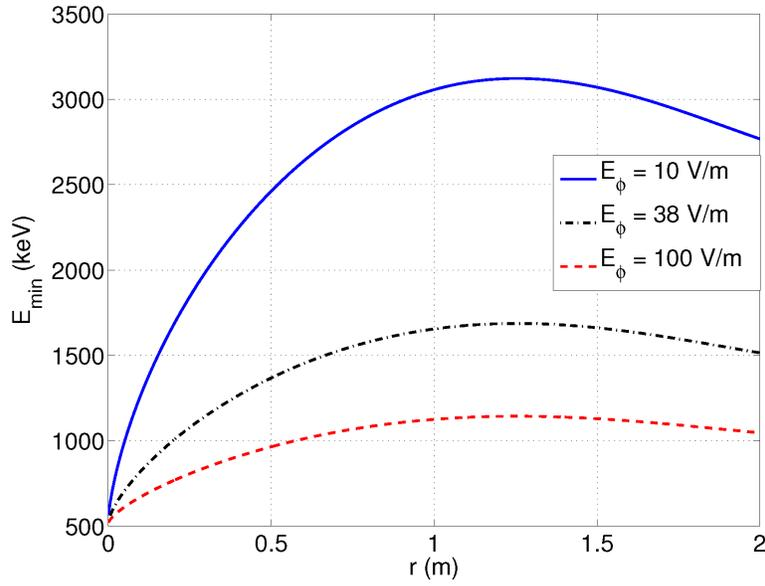
Figure 6.10: The minimum energy needed for the Ware pinch to be faster than the collision time, for the parameters  $E_\phi = 10$  V/m, 38 V/m and 100 V/m,  $n_e = 10^{20}$  m $^{-3}$  and  $R = 6.2$  m. The poloidal magnetic field is calculated from a current density profile with a total plasma current of  $I_p = 15$  MA.
