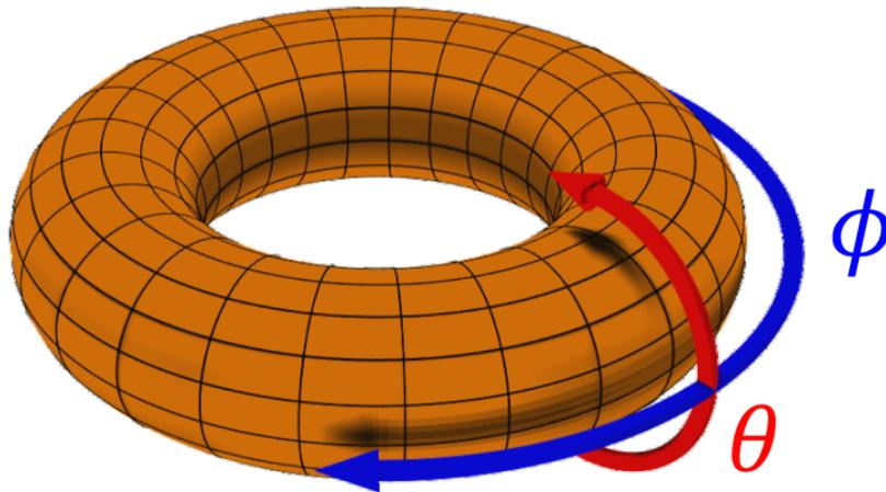
Figure 2.1: The toroidal ( $\phi$ ) and poloidal ( $\theta$ ) direction.
