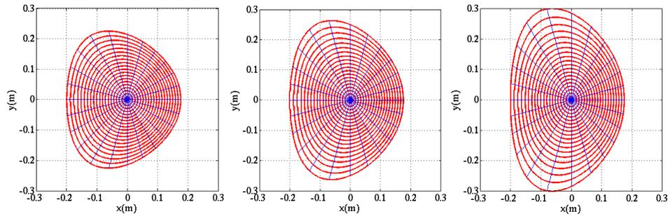
Figure 7.24: Magnetic geometry calculated by METIS for  $\kappa=1.2,1.4$  and  $1.6$ .
