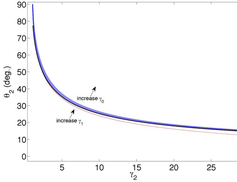
Figure 4.2: The dependence of the scattering angle of initial energies of the target electrons ( $\gamma_2$ ). Black line is  $\gamma_0 = 1, \gamma_1 = 10^5$ . For blue lines  $\gamma_0 = [1 : 0.01 : 1.1]$  and  $\gamma_1 = 10^5$ . Red line is  $\gamma_1 = 100$  and  $\gamma_0 = 1$ .
