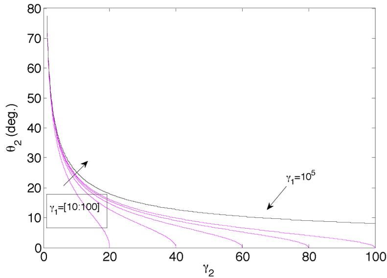
Figure 4.3: The scattering angle  $\theta_2$  at various initial energies of the primary electron ( $\gamma_1$ ) as a function of the energy of the initially slow electron ( $\gamma_2$ ). Here  $\gamma_1 = 10 : 20 : 100$  and  $\gamma_0 = 1$ .
