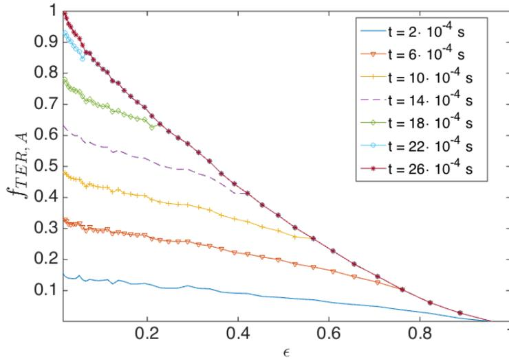
Figure 6.12: The radial distribution function of the trapped-electron avalanche, with  $E_\phi = 10$  V/m and  $B_\theta = 0.01$  T, calculated from the bounce-averaged knock-on operator implemented in the LUKE code.
