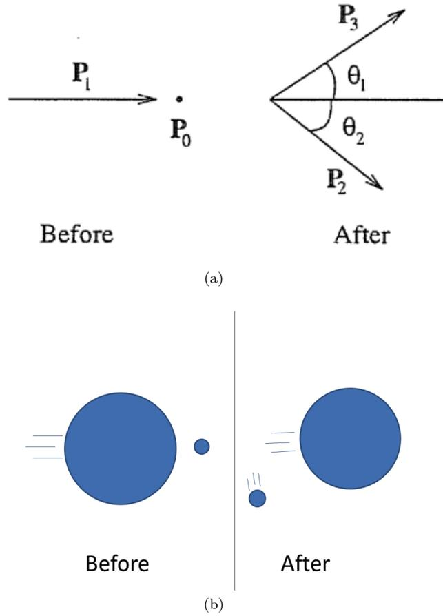
Figure 4.1: Illustration of close collisions between a relativistic electron and an electron at rest (a). Since the electron mass is proportional to the Lorentz factor  $\gamma$  the relativistic mass of the relativistic electron is much larger than the mass of the electron at rest (b).
