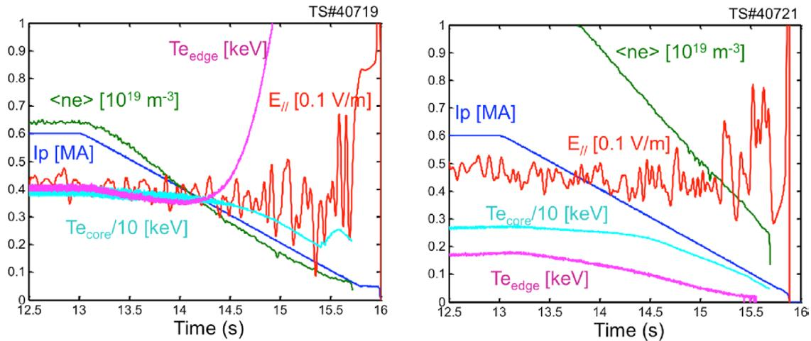
**Figure 10.** Possible signature of suprathermal electrons on the edge ECE chord ( $T_{e,edge}$ ) at around  $t = 14.5$  s are seen in the Tore Supra discharge 40719 (left). In a following discharge, with higher density (right), there is no sign of suprathermal electrons on the ECE measurements.  $E_{||}$  is the electric field strength,  $\langle n_e \rangle$  is the line averaged density and  $I_p$  is the plasma current.
