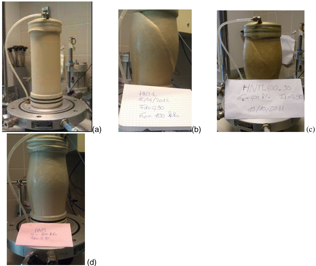
Figure 7 - Shear band formation inside the specimens. One or several bands are visible after testing (a) before testing (b) after testing under a confinement of 100 kPa, (c) after testing under a confinement of 400kPa (d) after testing under a confinement of 800kPa
