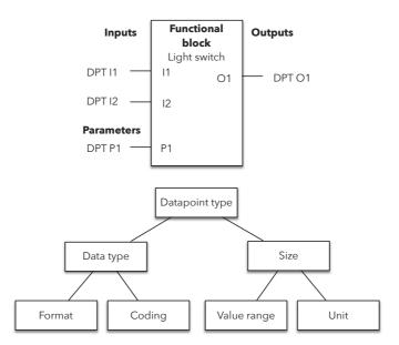
**Figure 2.8:** The upper part shows a functional block structure composed of datapoints acting as communication endpoints. The sub-components of a datapoint type including data representation and signification are depicted in the lower part.
