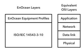
Figure 2.10: EnOcean protocol stack compared to the OSI model.
