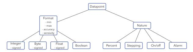
**Figure 4.24:** Datapoints are not predefined but can be composed by putting together different properties and classes. This approach offers much more flexibility compared to a finite set of definitions.
