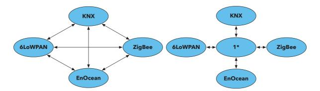
Figure 2.3: In the N-to-N approach (left) each device is able to understand the entire protocol set deployed in the building. The N-to-1\* approach (right) advocates the use of a shared protocol between all the technologies.
