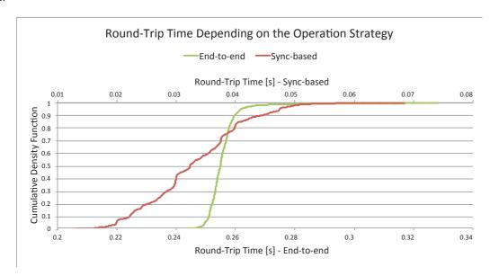
Figure 4.40: Round-trip time cumulative density function for the end-to-end and sync-based modes.
