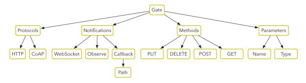
**Figure 4.19:** The gate properties describe how a resource should be consumed. This can serve as API documentation for humans building Web applications, but is especially intended to allow automatic mashup composition between machines.
