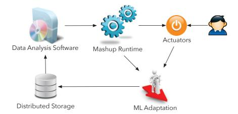
**Figure 4.51:** The adaptation layer will use actuators states and the actions performed by control scenarios to determine if an action was performed by the user. Conflicts will be notified in the distributed database so that the training process can refine its classes.
