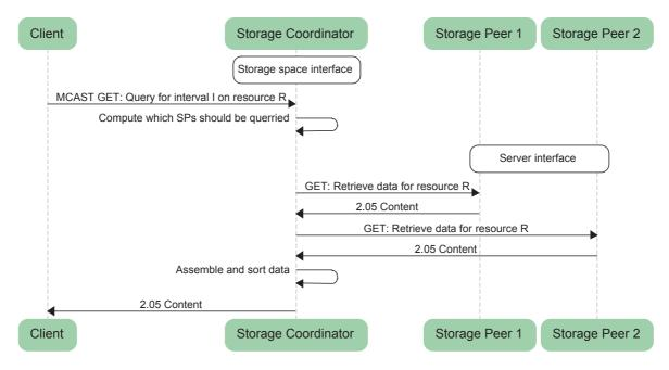
**Figure 4.29:** The sequence of exchanged messages for a client querying historical data with the interval of time I on resource R. The storage coordinator computes on which storage peers data should be retrieved to optimise the network traffic. It then assembles and returns it to the client.
