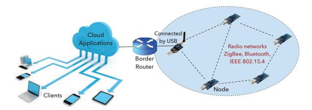
**Figure 2.1:** Example of a wireless sensor network where nodes are distributed among the physical environment for monitoring purposes. The communication is performed through low-power radio. The traffic directed to outward networks transits via a border router connected to the Internet.
