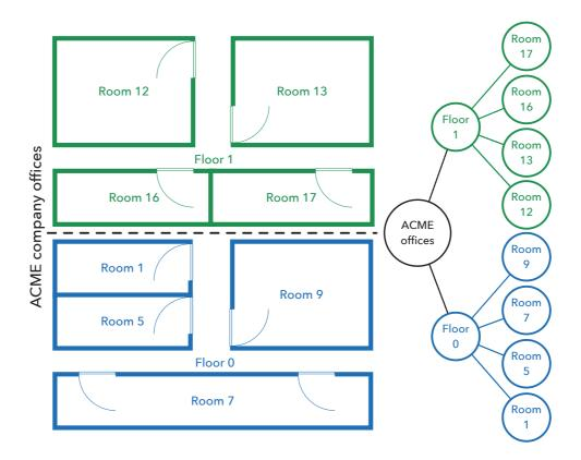
**Figure 4.10:** The building morphology composed of floors and rooms can be translated to a hierarchical tree structure. The creation of naming zones can subsequently rely on this organisational model.
