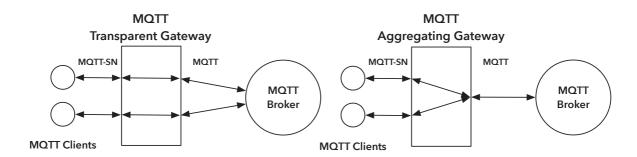
**Figure 3.5:** Gateways are required to interconnect the classical MQTT protocol with its sensor network optimised version. On the left the transparent gateway translates the protocol allowing end-to-end interactions. On the right the aggregating gateway only uses one connection to the broker and reformats the messages.
