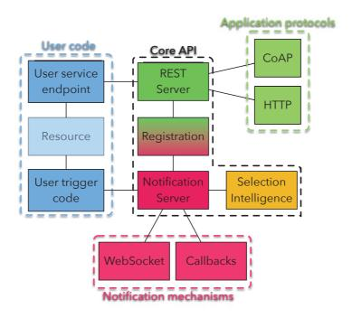
**Figure 5.8:** The Selection Intelligence module embeds the consumption models and is able to compute the energy of each notification technique. It is used by the Notification Server to decide which mechanism has to be used.
