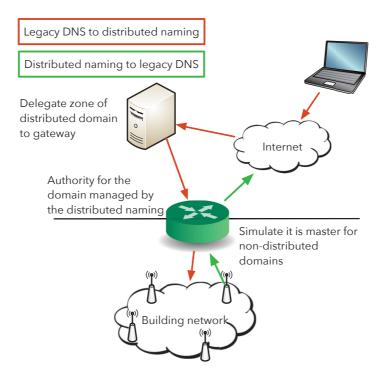
**Figure 4.15:** The building network using the distributed naming can be made compatible with the legacy DNS by introducing a gateway. Its role is to translate the requests and responses between the DNS protocol and the Web resources.
