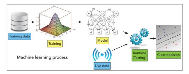
**Figure 2.4:** The machine learning process can be decomposed in distinct steps. The training part uses historical data as input and generates mathematical models. The runtime step (or testing step) applies the models on live data to perform the classification.
