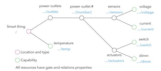
**Figure 4.23:** Resources on smart things can be represented with a tree like a file system. Collections can for this purpose regroup identical sub-resources identified by a number. In this concrete example we show how resources could be organised for a smart power strip.
