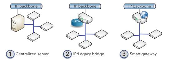
**Figure 4.25:** Connectivity with legacy building automation system can be achieved through several ways: a centralised server physically interfaced, a protocol bridge encapsulating telegrams in IP packets, or with a smart gateway mapping device functionalities to Web services.
