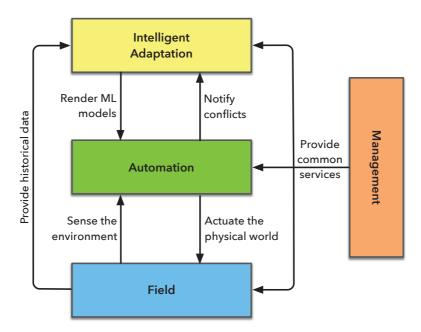
**Figure 4.2:** The interaction is not necessarily achieved by traversing all layers but must be seen as a set of services offering functionalities that can be easily reused among the other layers. The Management Level is positioned vertically as it offers essential common services such as naming or discovery.
