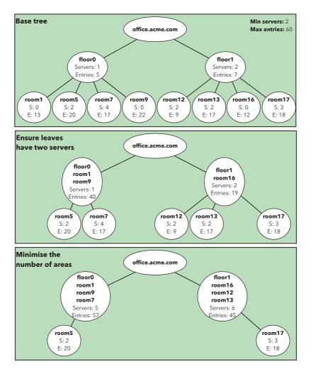
**Figure 4.12:** Example of the partitioning of a name tree with a minimum of 2 servers and a maximum of 60 entries per area. Each location corresponds to a single area in the first step, represented by the circles. The algorithm then ensures that all leaves meet the constraints. Finally, areas will be merged together whether possible to form combined circles.
