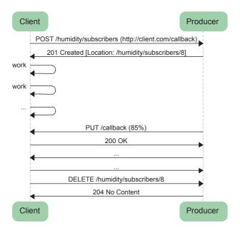
**Figure 4.4:** During registration, a client issues a POST request to the /subscribers sub-resource by including its callback in the payload. The producer responds with the Location option indicating the URI available for unregistration.
