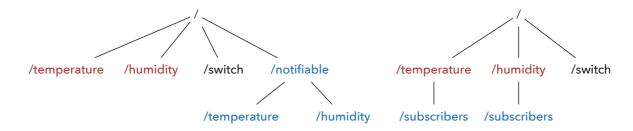
Figure 4.3: Two potential ways are available for a client to register for notifications. On the left part, a common resource (/notifiable) regroups all the resources offering notifications. Client will interact with these during registration. On the right part, each resource that supports notifications exposes a sub-resource (/subscribers) dedicated to registration. This latter way follows better the ROA style and is preferred.
