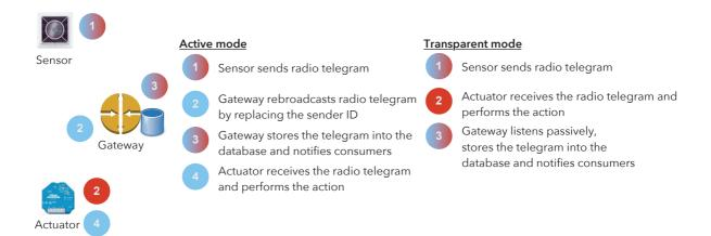
**Figure 5.3:** The EnOcean gateway can work according to two operation modes. In the *active mode*, actuators will only be paired with the gateway. In the *transparent mode*, sensors and the gateway will be paired with actuators.
