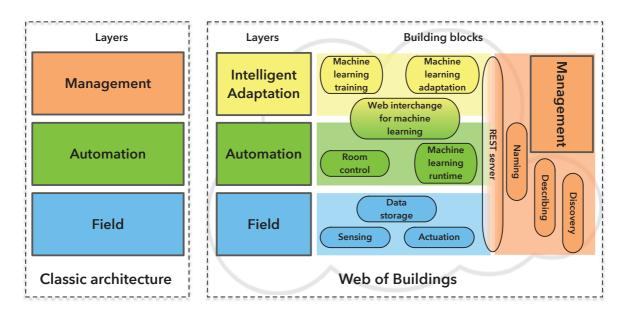
**Figure 4.1:** Comparison of the classic building automation layered architecture to our Web of Buildings contribution. Each layer can run separately and is composed of a set of building blocks facilitating the development of smart buildings.
