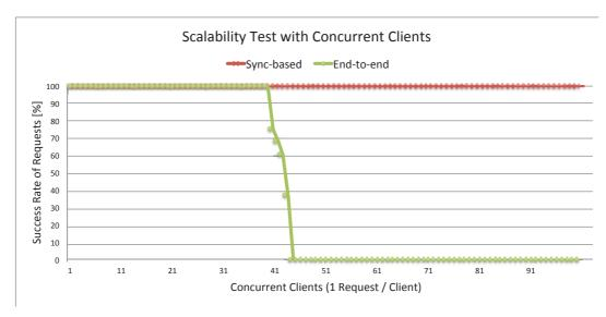
**Figure 4.42:** Comparing the scalability in terms of concurrent requests for the end-to-end and syncbased modes.
