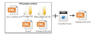
Figure 5.1: ETS project archive structure and XSL transformation.
