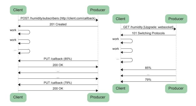
**Figure 3.3:** Sequence diagram of push techniques using HTTP. On the left the *HTTP Callback* transforms the client into a server exposing a callback resource to the producer. On the right HTTP is only used to initiate a *WebSocket* that will further switch to a bidirectional TCP connection.
