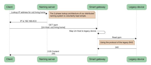
**Figure 4.26:** Clients reuse the same interaction concepts with legacy devices. The request will however be handled by a smart gateway mapping the Uri-Host to an address. Once having performed the action with the legacy device, it will put the result into the response.
