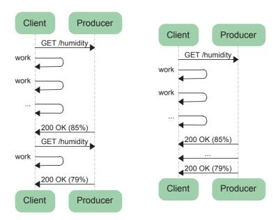
**Figure 3.2:** Sequence diagram of push techniques using HTTP. On the left *Long Polling* delays the HTTP response while there is no new value, therefore decreasing the polling frequency. On the right HTTP Stream keeps the connection open as long as possible, allowing to send HTTP responses only when new data is available.
