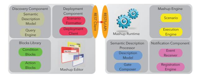
**Figure 4.47:** The mashup-based room control platform is divided into a series of components, each one performing a specific task. This architecture enables evolvability and allows components to be replaceable.
