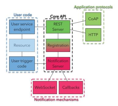
**Figure 4.5:** The hybrid REST server library is composed of several modules performing dedicated tasks in the overall architecture. This loosely coupled decomposition allows straightforward maintenance and also eases the addition of new modules.
