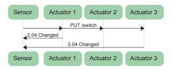
**Figure 3.8:** With CoAP group communication a client can simultaneously interact with remote endpoints. The sensor will be able to drive the actuators number 1 and 3 as they are in the same group. Devices that are not participating in this group will discard the request and do not respond (actuator 2).
