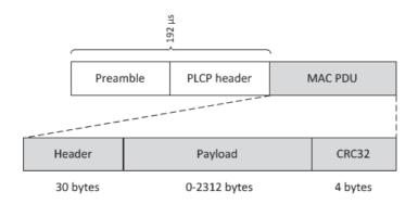
Figure 5.6: Composition of a 802.11 Wi-Fi frame taken from [279].
