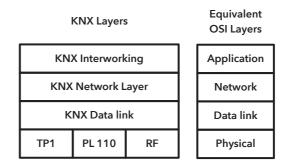
Figure 2.6: KNX protocol stack compared to the OSI model.
