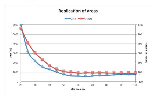
Figure 4.16: Total number of packets and data for 5000 random operations (add host, remove host, add server agent and remove server agent) on a simulated building structure composed of 180 rooms.
