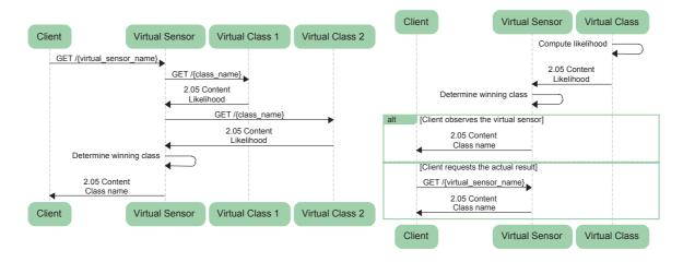
**Figure 4.38:** Clients can choose during the deployment of a Virtual Sensor the operating mode. On the left, with the end-to-end mode, the Virtual Sensor will sequentially retrieve likelihoods to determine the winning class. On the right, notifications are used with the sync-based mode to cache the winning class.
