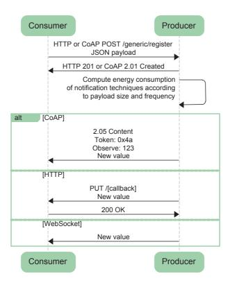
**Figure 5.7:** Clients register as consumers using a generic service that is either available over CoAP or HTTP. The notifications will then be sent according to the most appropriate notification mechanism.
