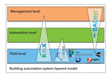
**Figure 2.5:** Building automation systems are composed of three layers. The field level gives access to devices functionalities while the automation level implements control strategies (control loops and rule sets). Finally the management level offers configuration interfaces for commissioning and other enterprise-level tasks.
