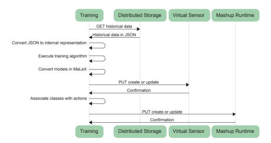
**Figure 4.49:** The machine learning training process is positioned on top of other levels. It retrieves the needed historical data from the in-network cloud storage. Once the models are trained, they can be deployed as Virtual Sensors. Furthermore, the training process can automatically define control scenarios in terms of mashups.
