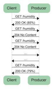
**Figure 3.1:** Sequence diagram of notifications between a client and a smart thing producing data. It follows the traditional HTTP pull interaction where the client constantly sends a request to gather the latest measurement.
