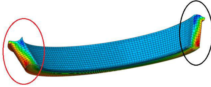
Fig. 6:9 Displacement contour under lateral load (half of the rubber component)
