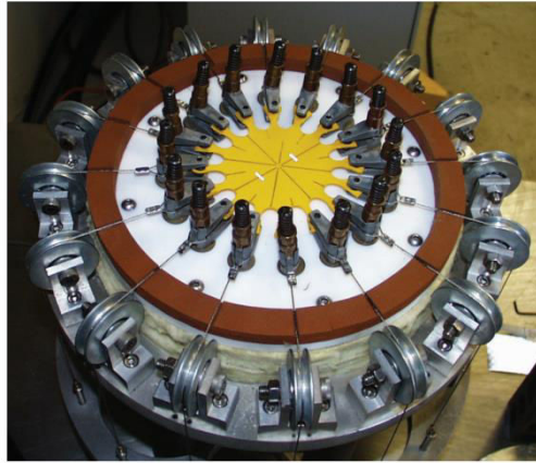
Fig. 4:2 Equal-biaxial tension test
