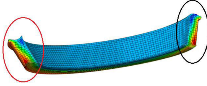
Fig. 6:9 Displacement contour under lateral load (half of the rubber component)
