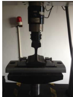
(a) The compressed type fastening system (b) The shear type fastening system
