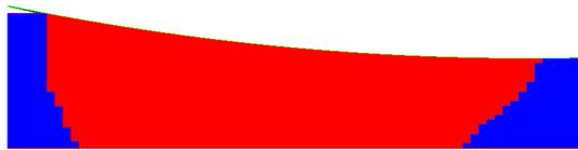
Figure 4.11: Case 2 - Hot finishing first stand. Plastic deformation area by *Lam3-Tec3*.
