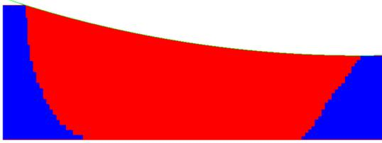
Figure 4.9: Case 1 - Hot roughing mill. Plastic deformation area by *Lam3-Tec3*.
