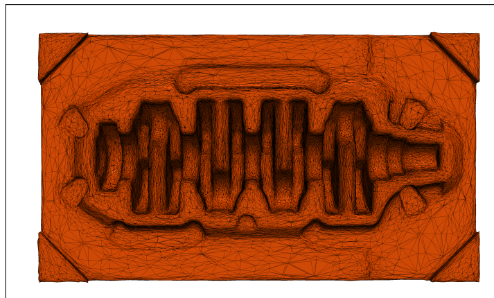
Figure 4.8: Mesh projected on the zero iso-value of the upper tool
