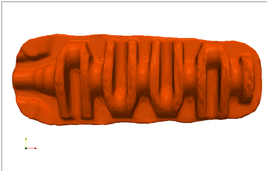
Figure 4.9: Geometry of the crankshaft at t \approx 0.9 s
