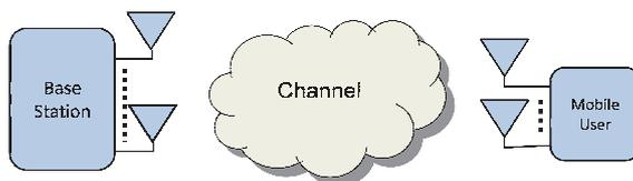
FIGURE 2.1 – Outage-limited channel model - no CSIT
