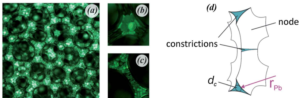
Fig. 1 Pictures showing foamy suspensions, (a) first layer of bubbles at the container wall. Fluorescent particles have been used in order to reveal the homogeneity of the sample over several bubble layers into the bulk. Bubble and particle sizes are respectively 660\ \mu\text{m} and 80\ \mu\text{m} ( \lambda = 1.7 ). (b) Detail from the left picture (in the bulk, not at the wall). (c) Same situation except for the particle size ( 40\ \mu\text{m} , \lambda = 0.85 ). (d) Sketch of the foam network showing the nodes and the constrictions; r_{pb} is the characteristic radius of curvature of the foam network and d_c is the diameter of passage through constrictions.
