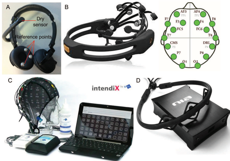
Fig. 2.2: Illustration of different BCI products. (A) Neurosky's Mindset. (B) Emotiv devices and its montage of electrodes. (C) G.tec's IntendiX. (D) Neural Impulse Actuator.
