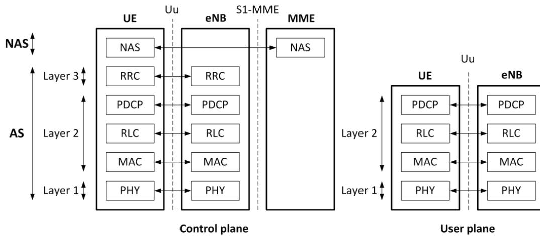
Figure 2.4: LTE Protocol stack [11]
