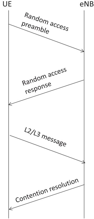
Figure 3.3: Contention based random access in LTE
