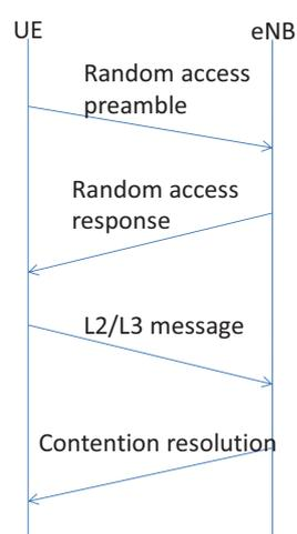
**Figure 2.7:** Contention based random access in LTE
