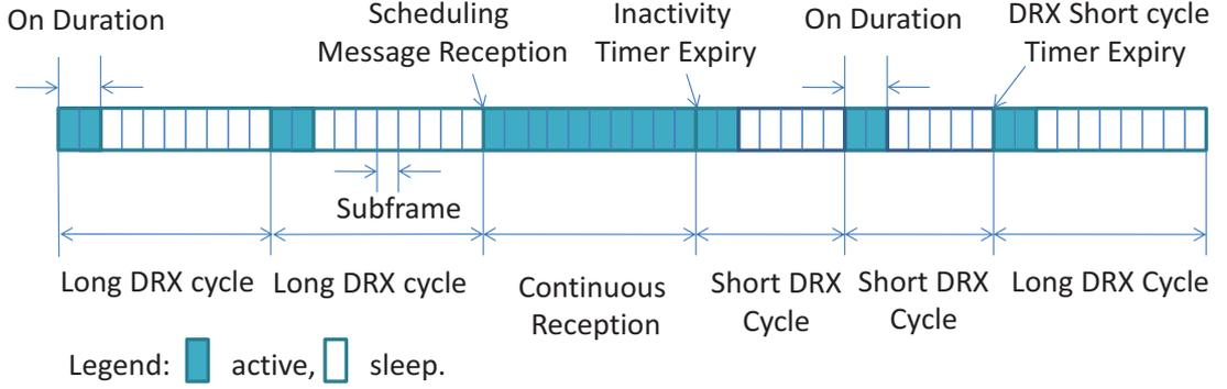
Figure 5.1: DRX procedure in LTE [9]
