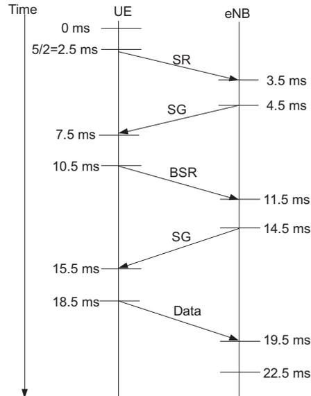
**Figure 2.9:** Uplink packet scheduling in LTE
