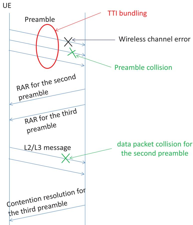
**Figure 3.17:** contention based random access with TTI bundling
