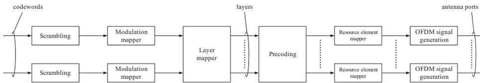
Figure 2.6: Overview of downlink physical channel processing [13]
