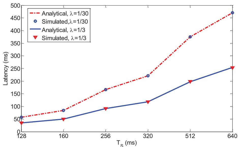
(a) Latency under different short DRX cycle,  $T_L = 2T_S$
