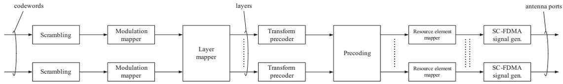
Figure 2.5: Overview of uplink physical channel processing [13]
