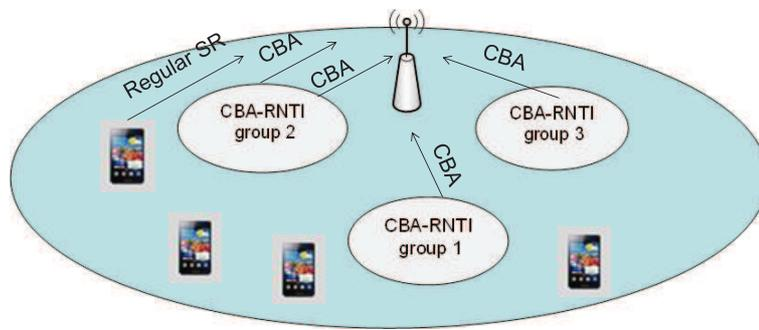
Figure 4.2: Uplink channel access with contention based access
