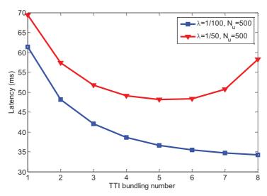
Figure 3.22: Latency under different TTI bundling number
