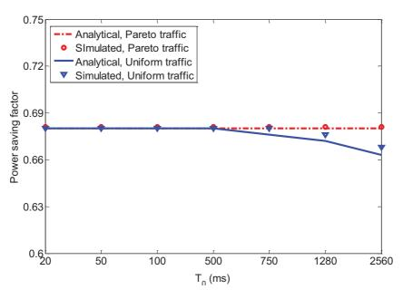
(b) Power saving factor under different Inactivity timer
