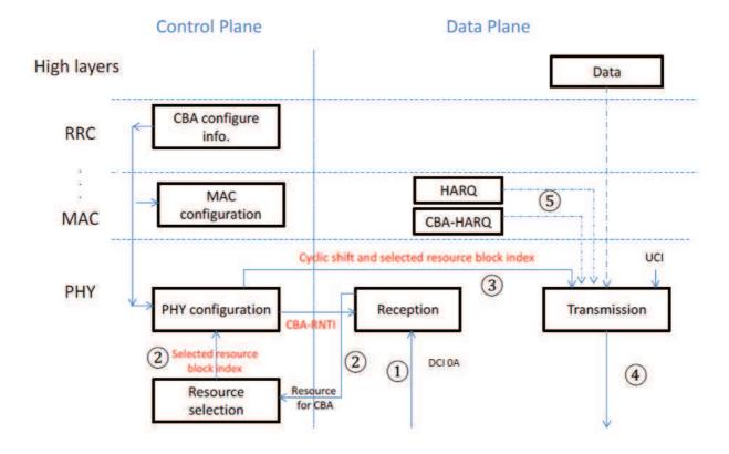
Figure 4.10: CBA architecture at UE side
