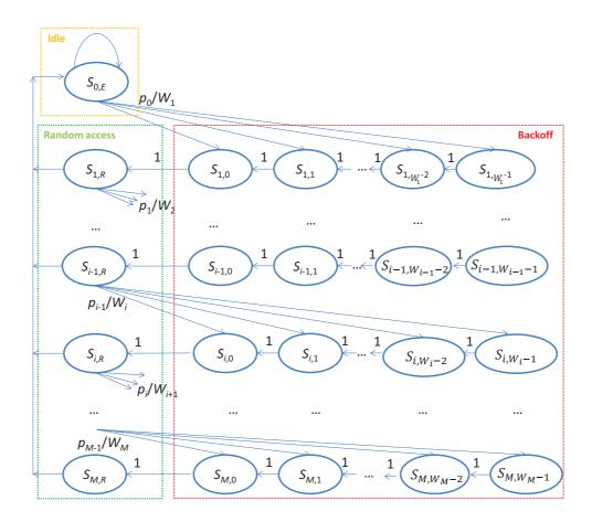
Figure 3.18: Semi-Markov process model for random access with TTI bundling
