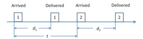
Figure 5.10: packet delivery procedure with DRX
