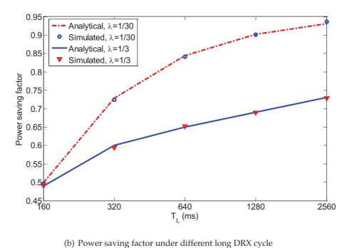
Figure 5.9: DRX performance under different long DRX cycle
