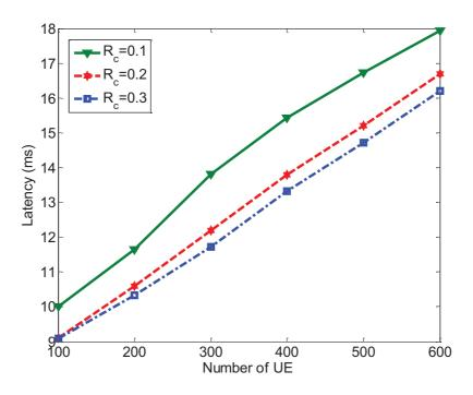
**Figure 4.15:** Effect of  $R_c$  on the CBA performance
