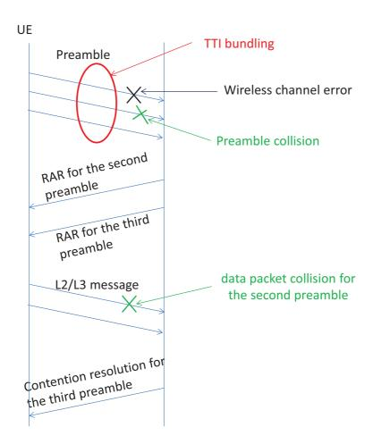
Figure 3.17: contention based random access with TTI bundling
