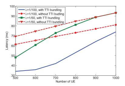
Figure 3.21: Latency comparison with and without TTI bundling
