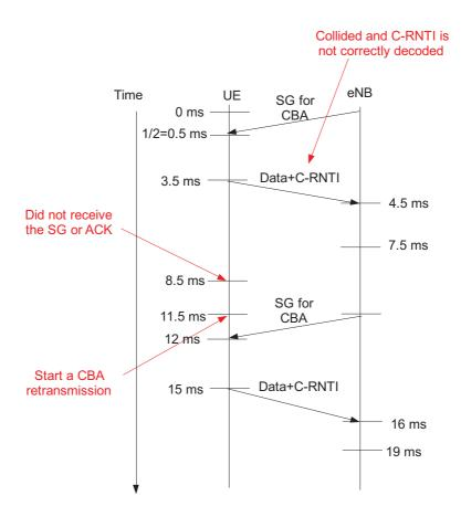
Figure 4.5: Contention based access with retransmission
