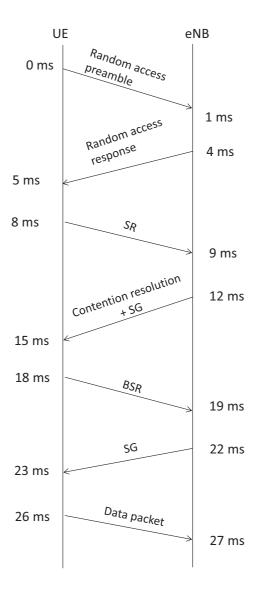
Figure 4.1: Data packet delivery with random access
