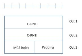
Figure 4.7: Control element for MCS and C-RNTI
