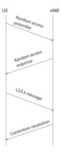
Figure 3.3: Contention based random access in LTE
