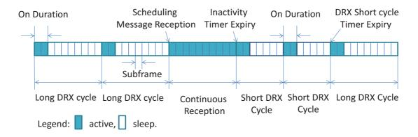
Figure 5.1: DRX procedure in LTE [9]
