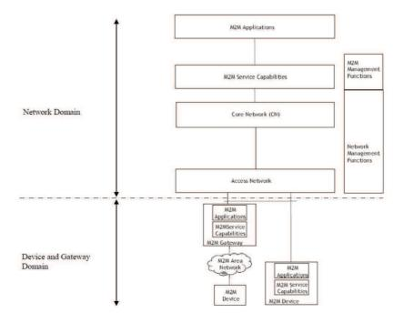
Figure 2.11: High level architecture for M2M [23]
