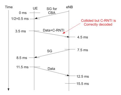
Figure 4.4: Contention based access with collision detection
