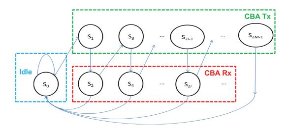
Figure 4.12: Markov chain model for contention based access
