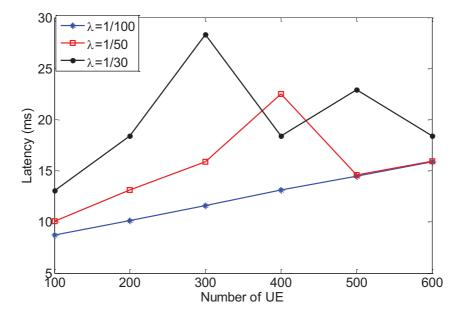
Figure 4.19: Latency of CBA resource allocation method
