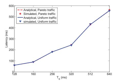
(a) Latency under different short DRX cycle,  $T_L=2T_{\cal S}$
