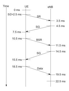
Figure 2.9: Uplink packet scheduling in LTE
