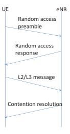
Figure 2.7: Contention based random access in LTE
