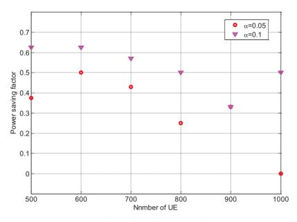
**Figure 3.25:** Power saving factor for different  $\alpha$  with Algorithm 1,  $\lambda = 1/100$
