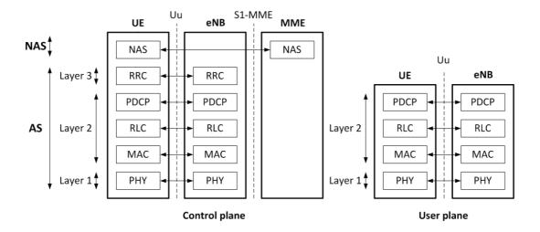
Figure 2.4: LTE Protocol stack [11]
