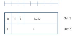
Figure 4.9: Subheader for CBA control element
