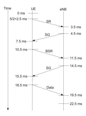
Figure 4.6: Uplink packet scheduling in LTE
