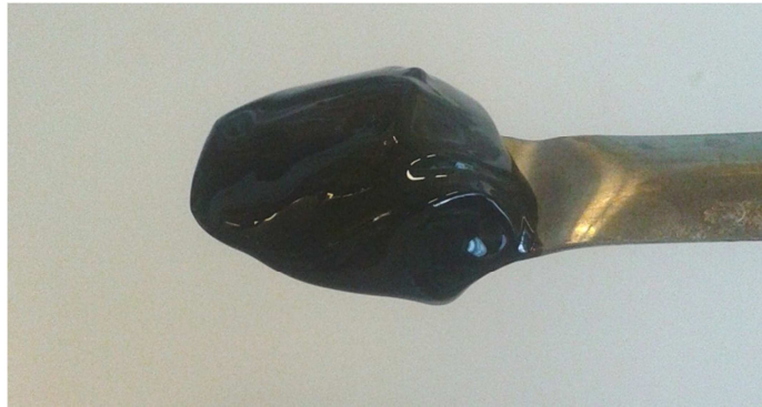
Figure 1.2. Waxy crude oil sample. When below its WAT, as in this image, it exhibits a yield stress.
