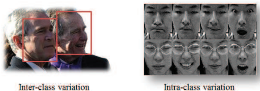
Figure 2.5: Inter and intra class variation in face recognition problems. Left: inter-class variation could be small between persons with biological ties. Right: Intra-class variation could be significant due to different poses, illumination, and expression.
