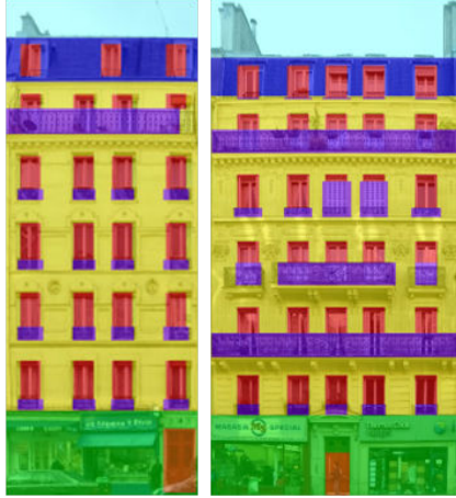
Figure 2.2: Semantically incorrect facade segmentation that can result from applying locally optimal corrections [33], for example, aligning pairs of lines that are sufficiently close. Note the balcony ending in the middle of a window in the left image, and the excessively large balconies in the right image. These artifacts result from not enforcing hard constraints on the resulting segmentations.
