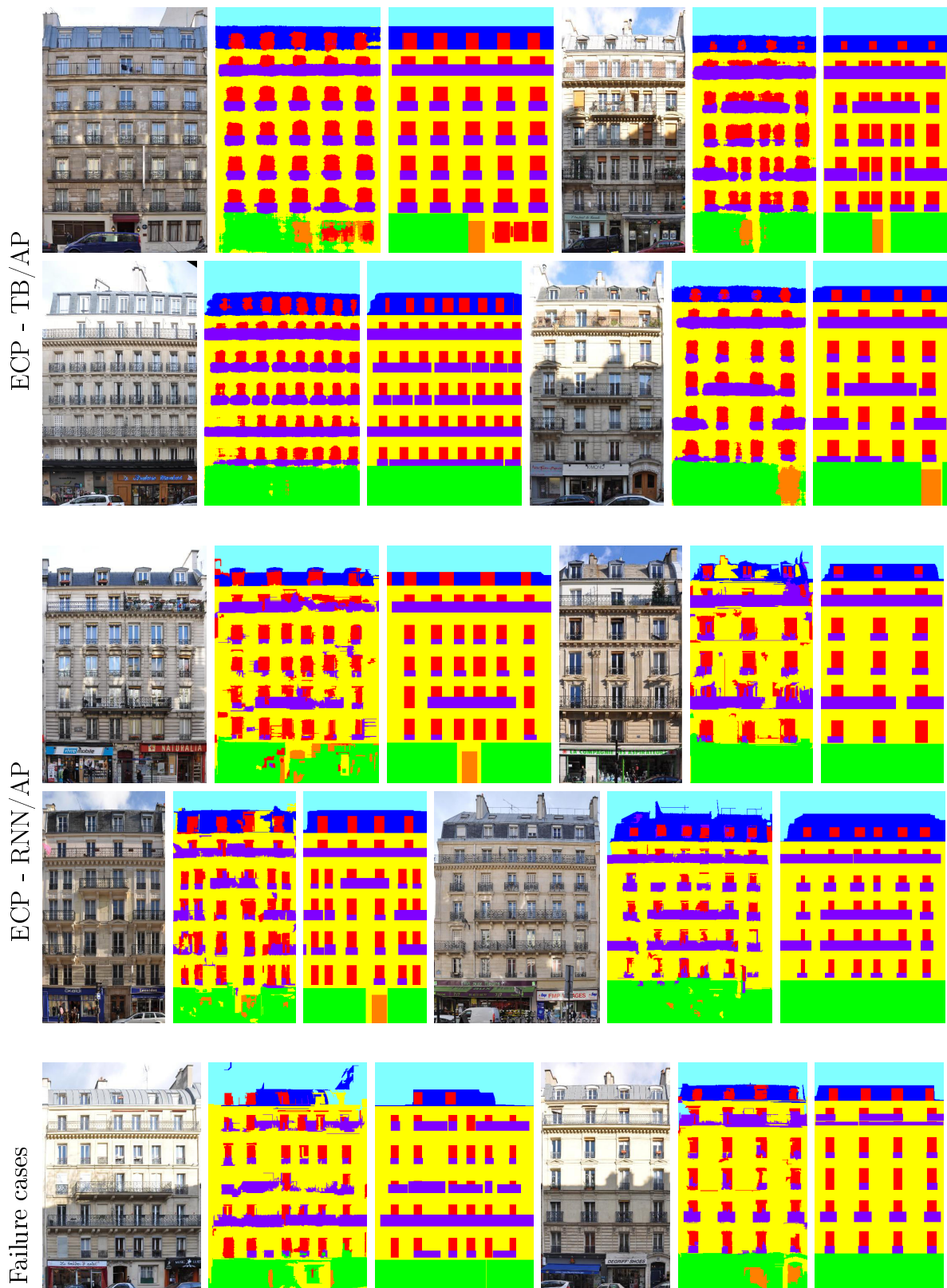
Figure 5.8: Example triplets of parsing results with adjacency patterns: original image (first of each three images), result of per-pixel classification (second image), parsing result (third image). The first two rows present results obtained using the TextonBoost potentials, the third and fourth rows contain results obtained using RNN. The last row contains examples of inaccurate segmentations (note that in the last segmentation there is a very thin line of windows between the two topmost balconies).
