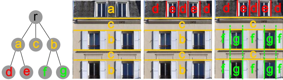
Figure 4.1: The shape prior consists of a hierarchy of rectangle classes (image 1 on the left) and a table of pairwise potentials for each nonterminal node (not shown here). Each image (2-4) shows the substitution of all rectangles of a particular class with any number of rectangles of any child classes. The class denoted by r , corresponding to the root of the hierarchy, represents the whole image. The remaining classes are: a -attic, b -floor, c -wall between floors, d -roof, e -attic window, f -wall between windows, g -window. The two-dimensional alignment of windows in the facade (but not attic windows) is enforced by the requirement that all floors are split in the same way.
