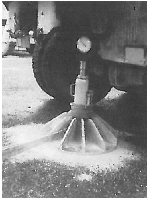
Fig. A.14 Plate load test – Westergaard type (Cassan 1988)
