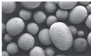
Electron micrograph of Micronal DS 5038 X. The powder particles consist of agglomerated microcapsules.
