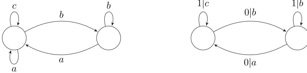
Figure 6.1: A sofic automaton of a channel C (left) and a (\{0, 1\}^*, C) -encoder (right)
