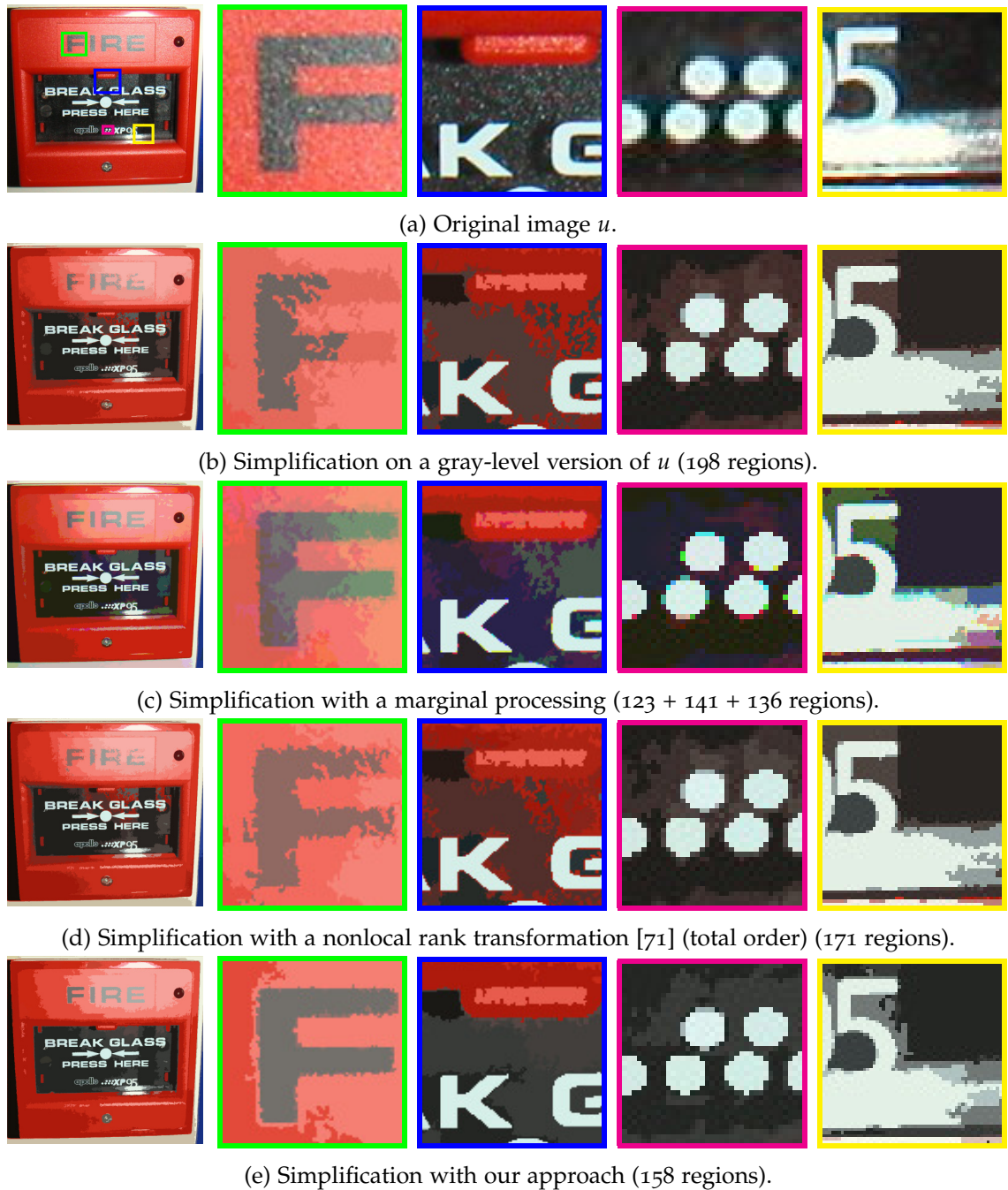
Figure 43: Simplification issues with “standard” color image processing. (b) and (d) show leakage problems with total ordering. (c) illustrates the false color problem due to marginal processing. (e) shows that the MTOS retrieves correctly the main content of the image while preventing false colors.
