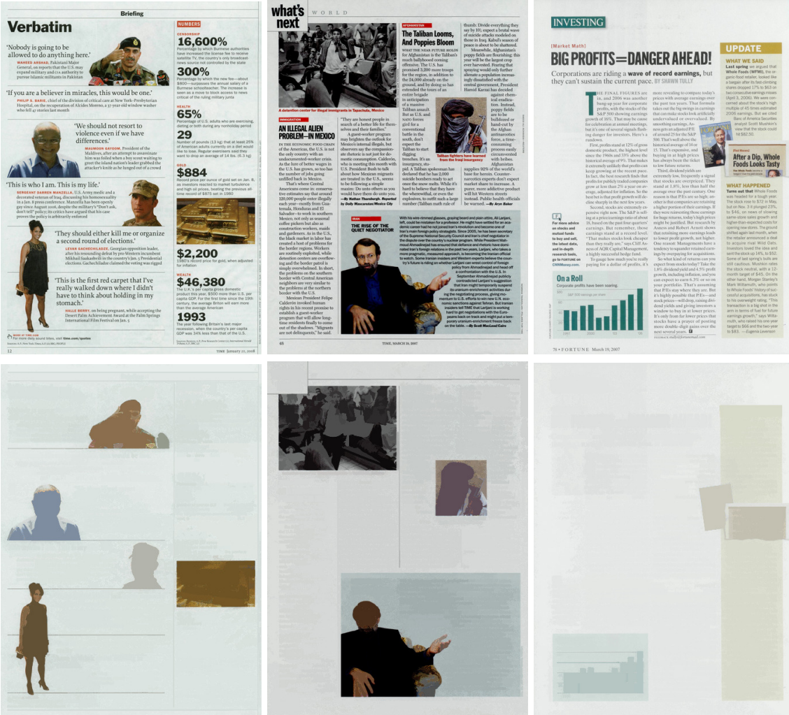
Figure 49: Simple filtering for document layout detection. Top row: original images; bottom row: results of grain filters.
