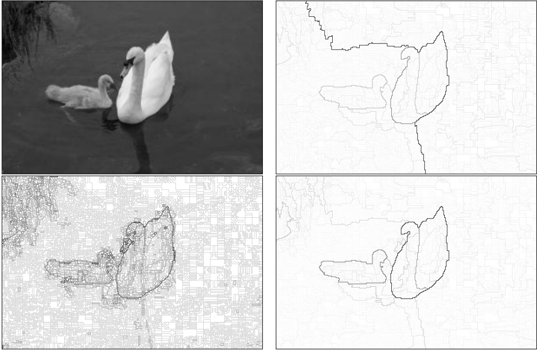
Figure 16: Hierarchies of watershed. Top left: original, top right: flooding by dynamics, bottom left: flooding by area, bottom right: flooding by volume. Hierarchies are represented through their saliency map.
