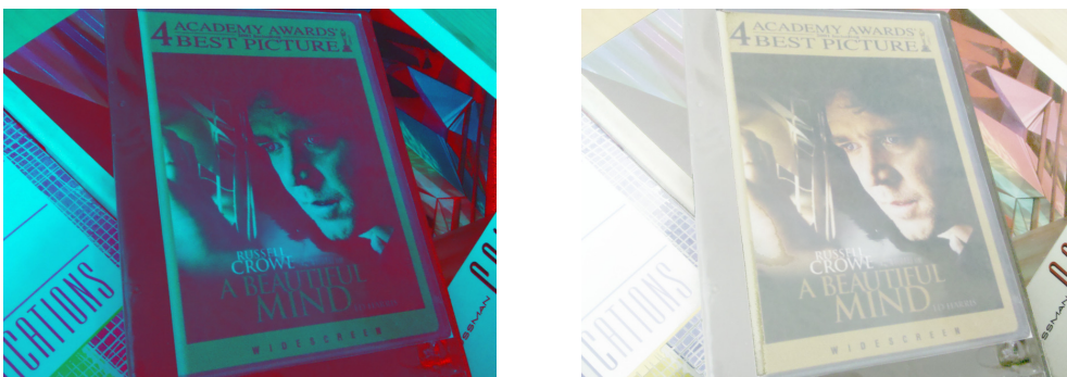
(b) On the need for contrast change/inversion invariance. The original image has been subjected to a global marginal inversion and/or change of contrast (left) and to a local change of contrast (right). They give the same MTOS, so the same level lines depicted in (a).
