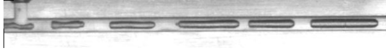
Figure 6.21 – Pictures of the steady regimes obtained with a peristaltic pump for emulsions and \frac{Q_g}{Q} \simeq 3 .
