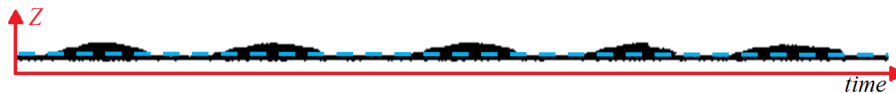
Figure 6.14 – Portion of a spatiotemporal diagram of bubble production (five bubbles). The cyan dashed line is used to obtain the signal values. Black and white area correspond to gas and yield-stress fluid respectively. The maximum height of the gas thread is 500 \mu\text{m} , each period lasts \simeq 11.5 s.
