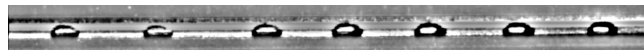
Figure B.3 – Side view of six bubbles produced in a T-junction ( R = 1 mm; L = 10 cm) filled with carbopol ( \tau_y = 75 Pa).
