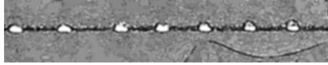
Figure B.2 – Top view of six bubbles produced in a T-junction ( R = 1 mm; L = 10 cm) filled with carbopol ( \tau_y = 75 Pa). We distinguish the egg-like shape of bubbles.
