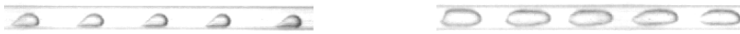
(a) Picture of five bubbles at large Bingham number ( Bi > 1 ). (b) Picture of five bubbles at small Bingham number ( Bi < 1 ).
