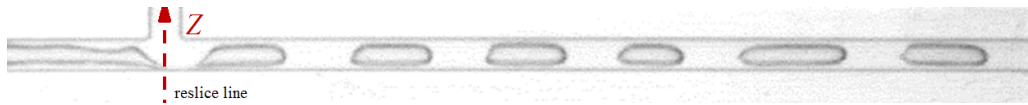
Figure 6.13 – An image taken during bubble formation in a steady state for R = 1 mm.
