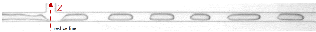
Figure 6.13 – An image taken during bubble formation in a steady state for R = 1 mm.
