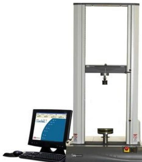
FIGURE 2.9 – Machine de force
