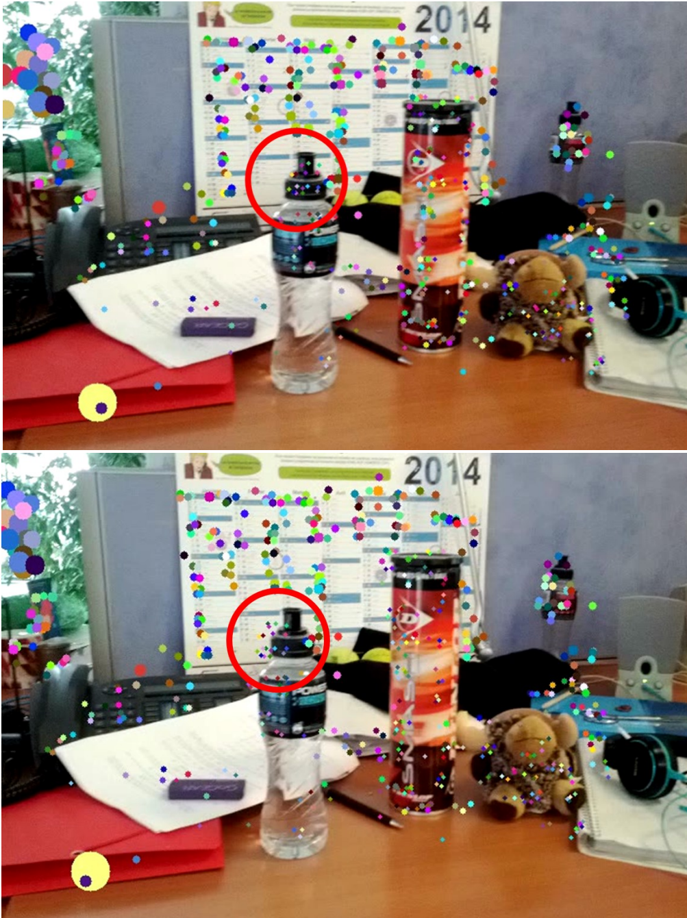
Figure 4-5: A change of direction occurs, leading to the UKF dynamic model prediction to offset a bit the localization. Top displays a frame in the sequence where the model is well tracked, bottom shows that right when the changes of direction happens, the model is not well mapped on the scene.
