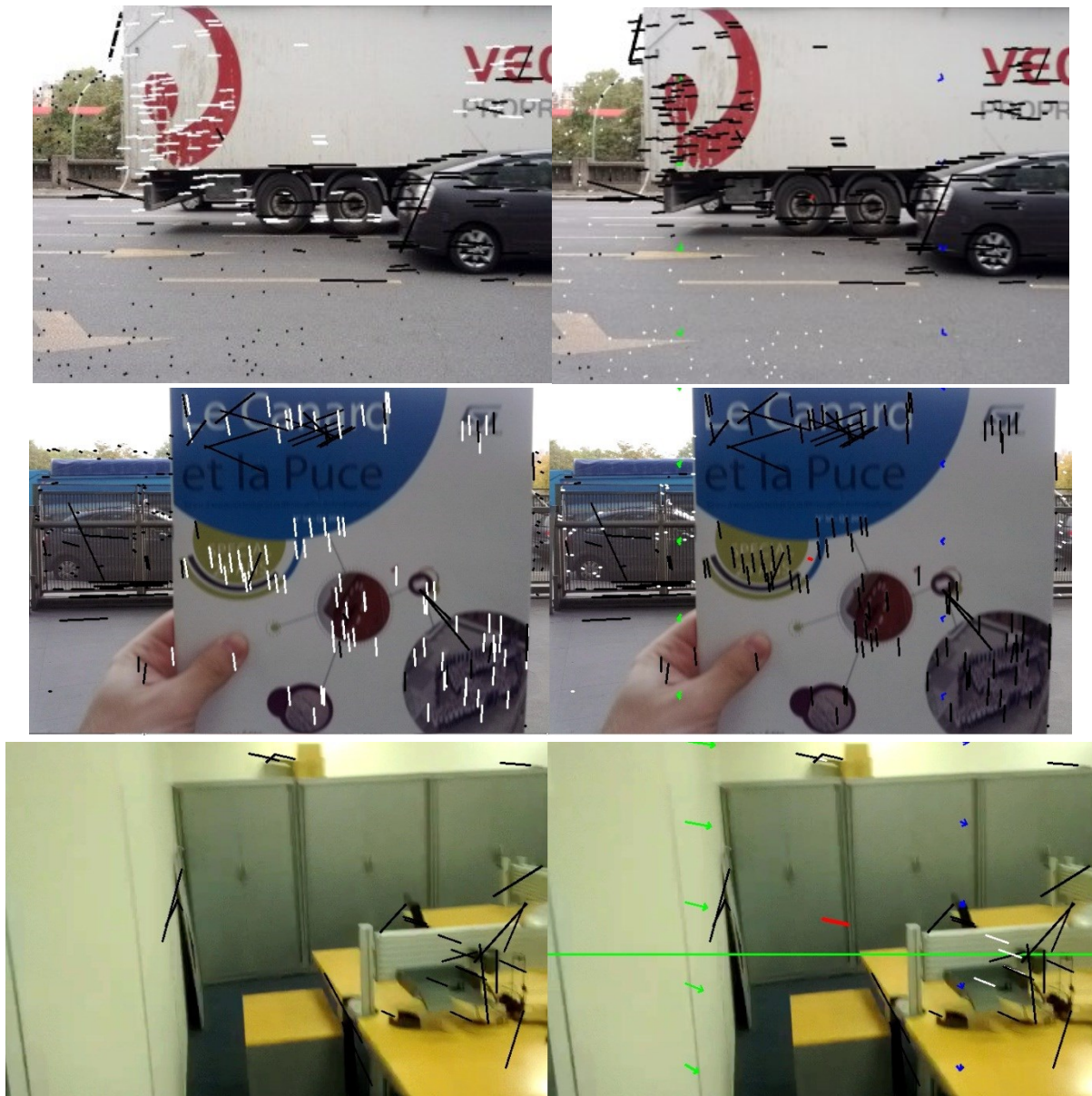
Figure 3-9: A few examples of test sequences by the preemptive RANSAC (left) and presented Hybrid RANSAC (right)
