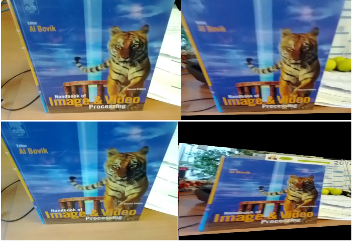
Figure 2-16: Two frames of the sequence (left) and the first frame warped in the perspective found by IBRIEF matches and RANSAC algorithm. In the first frame (353), the pitch is low-enough to allow a good performance by the technique. In the second one (375) the pitch is too high for the approach.
