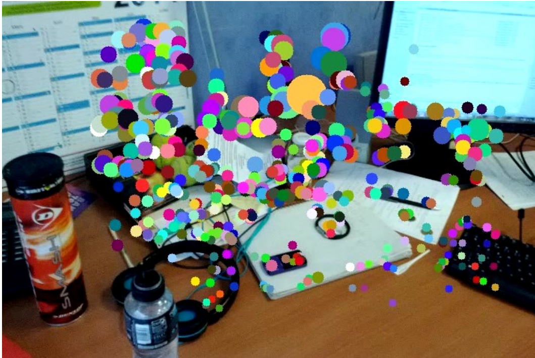
Figure 4-4: A 3D map computed with the 7-point RANSAC algorithm. The smaller the circle is displayed, the closest is the point.
