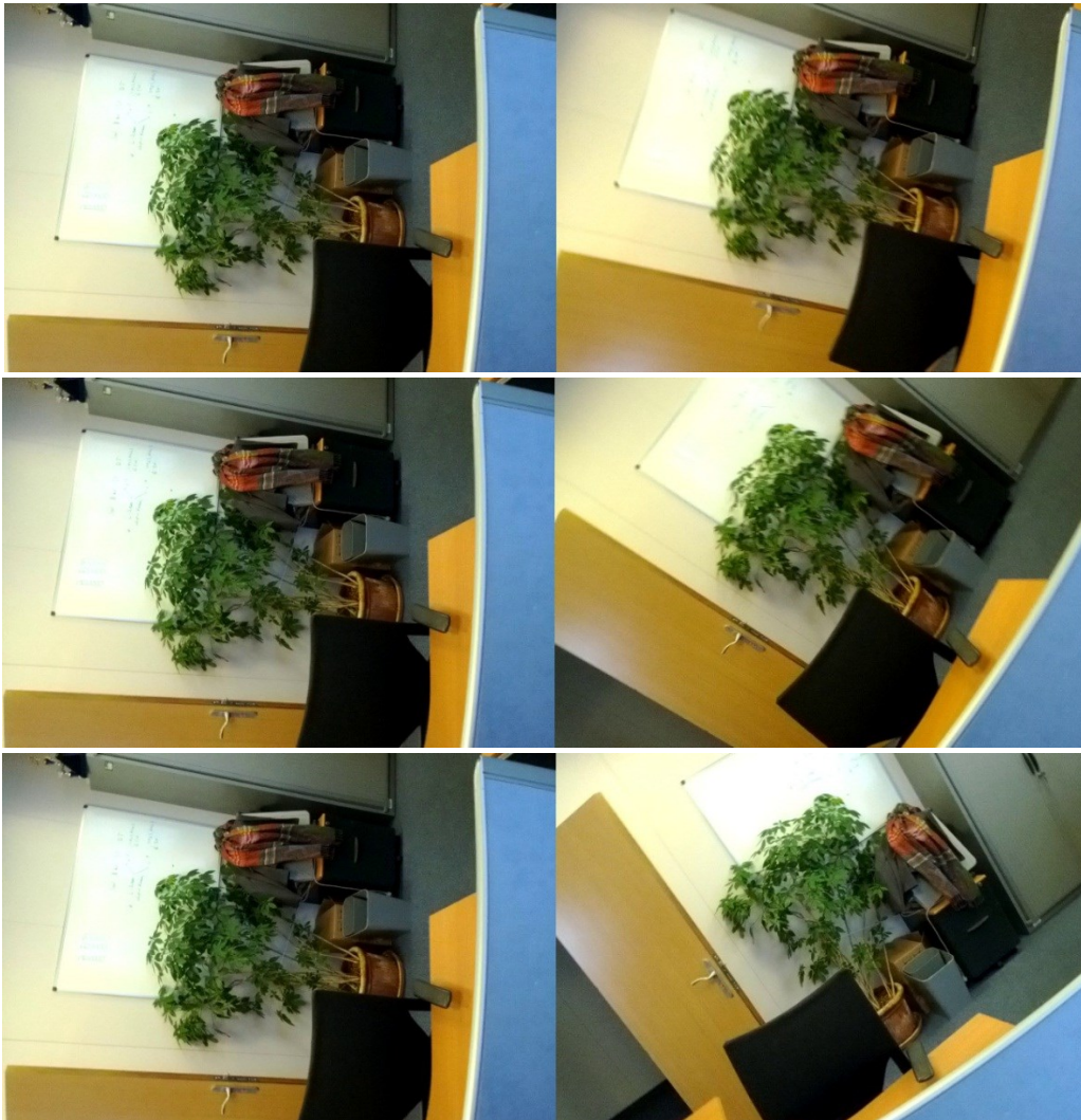
Figure 2-11: A few frames extracted from the first sequence: we match the first frame (left) with other frames in the sequences (right). This sequence consists in a progressive roll motion.
