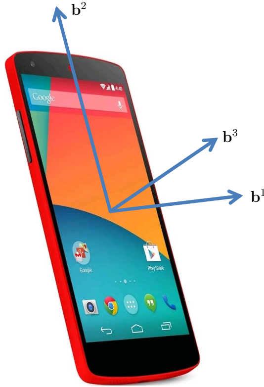
Figure D.15: The body-frame is aligned with the principal axis of inertia of the smart-phone.
