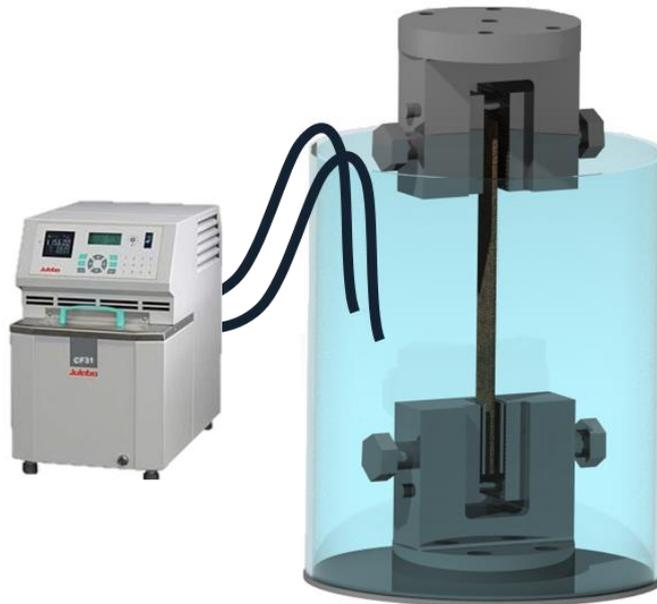
Figure II-VIII Mechanical-hydrothermal set-up.
