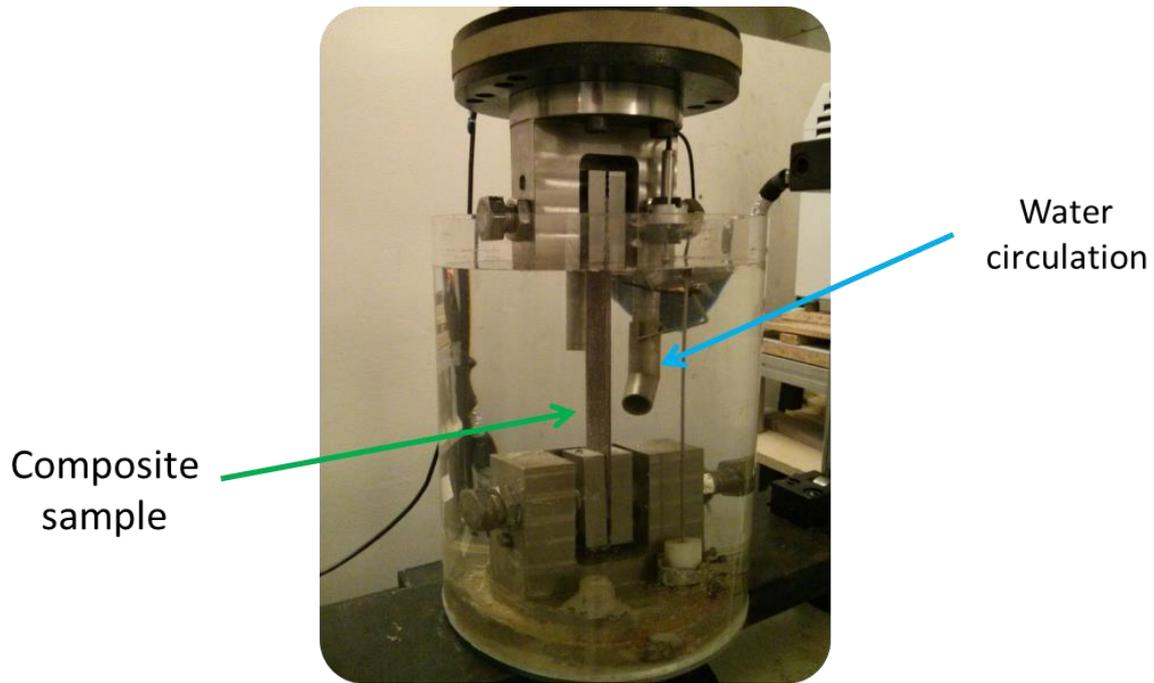
Figure II-XIII Configuration of the mechanical-hydrothermal characterisation for flax fibre composites.
