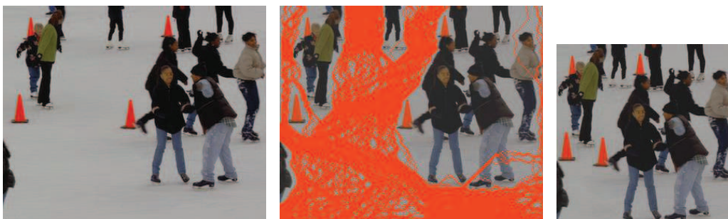
Figure 15 Illustration of the group of seams for ice. From left to right: original image, original image with the seams in orange, reduced image.
