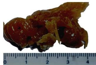
**Figure I. 1: Browning in blend of LDPE + (E-C) processed at 160°C.**
