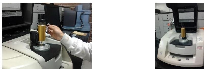
**Figure 2.4:** ATR accessory used to collect spectra of liquids.
