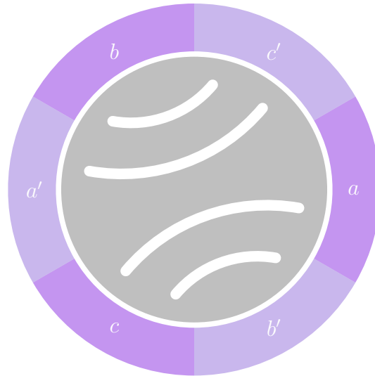
Figure 1.2 – Schematic transverse representation of a three-phase one-pole-pair SynRM
