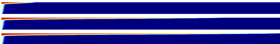
Figure 5.16 – Gas saturation map in range [0, \max(S_g)] : \max(S_g) = 0.7 at 120 d (top), \max(S_g) = 0.73 at 16 y (center) and 30 y (bottom), [100, 2500] m.
