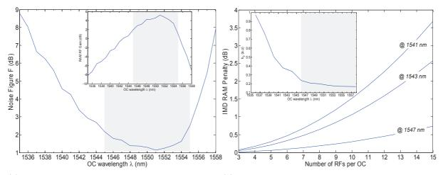
(a) Noise figure of the EAM vs.  $\lambda$  at 10mW input optical(b) IMD penalty at different OCs assuming an equally spaced power. Inset: Modulator RF Gain. RF mapping. Inset:  $3^{rd}$  order RAM non-linearity parameter
