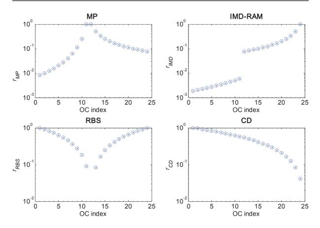
Figure 6.2: OCs ranking for MP, IMD-RAM, RBS and CD impairments. A WDM pool of 24 OCs with 1 nm channel spacing in the C-band is assumed. Y-axis is log-scaled.
