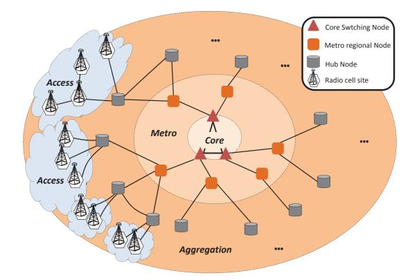
Figure 3.1: Generic model and subcomponents of the mobile backhaul.
