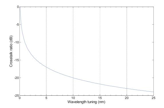
$\frac{\text{Figure 4.10: Crosstalk coefficient of a uniform BFG vs. wavelength tuning.}}{\text{A uniform FBG model is used to compute reflected and transmitted signal spectra. A detuning of 1 nm from the reflected wavelength causes a crosstalk coefficient of -10 dB. To minimize the effect of heterdyne crosstalk, active optical channels should be enough spaced.}}$
