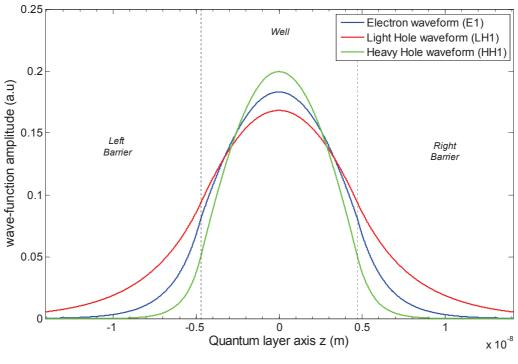
Figure A.2: Wave-functions of the QW-EAM for 1550 nm incident light under 0 V
