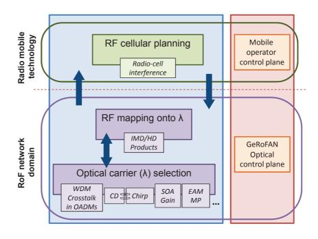
Figure 5.1: The cross-layer architecture of the GeRoFAN-CP.
