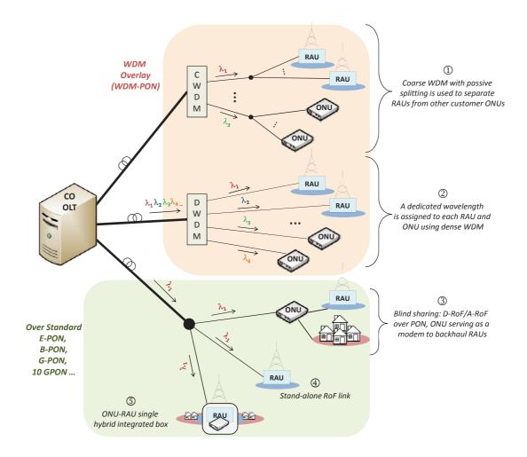
Figure 3.9: Different RoF-fixed optical broadband integration schemes.
