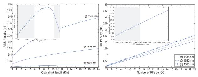
(c) RBS penalty at different OCs. Inset: RAM RF Gain. (d) CD penalty with 10 km fiber. Inset: CD coefficient vs.  $\lambda$ .
