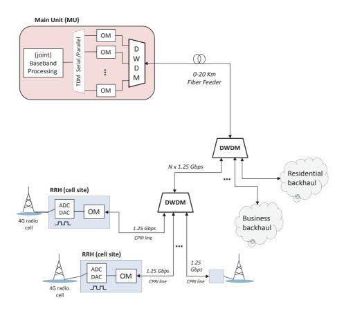
Figure 7.2: D-RoF WDM-PON network architecture
