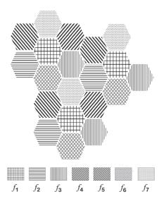
Figure 5.8: A 7 frequency reuse planning.
