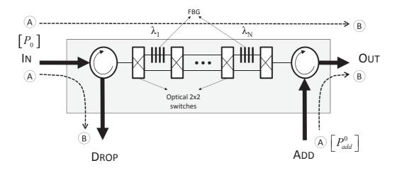
Figure 4.8: ROADM Structure used for GeRoFAN
