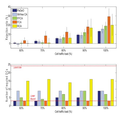
Figure 5.15: PaGeO vs. Other Policies (RCA, FCA, FFCA, IM-free CA) at different traffic loads. Error bars stand for deviation from the mean value. Negative rejection ratio means excess capacity more than the required load.
