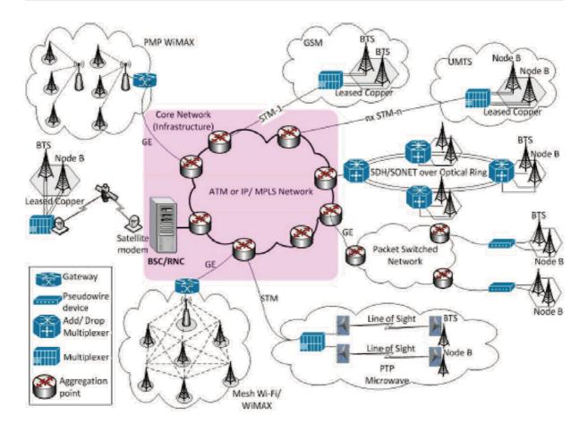
Figure 3.2: Traditional/emerging backhaul technologies: A big picture view [102].
