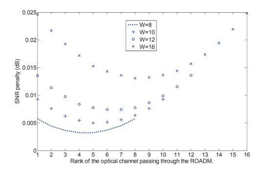
Figure 5.5: SNR penalty when passing through the ROADM.
