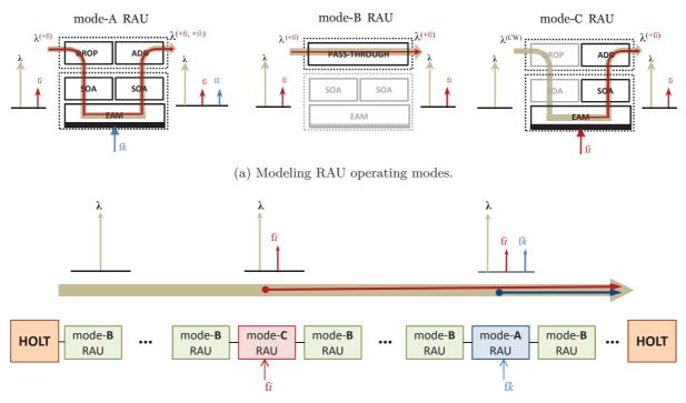
(b) An example of lightpath build as cascaded RAUs as seen by RF  $f_i$ .
