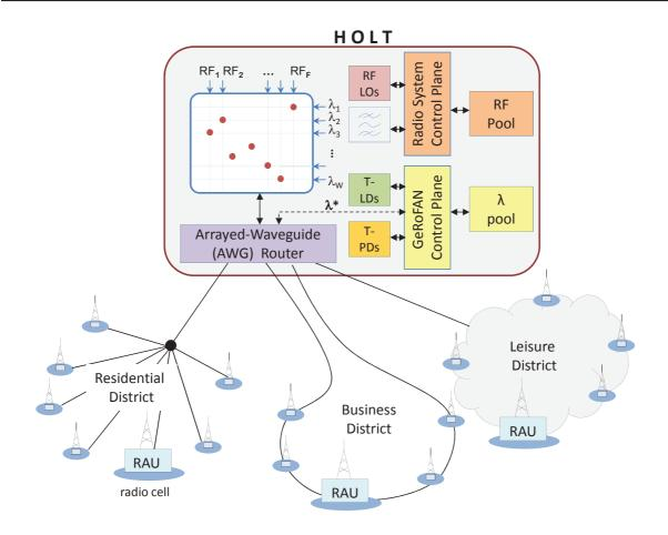
Figure 3.16: Generic Radio-over-Fiber Network Architecture.
