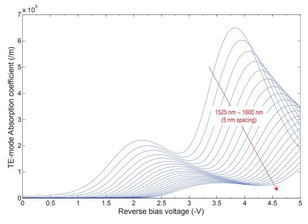
$\frac{\mbox{Figure A.5: MQW-EAM absorption coefficient profile from 1525 $nm$ to 1600 $nm$.}}{\mbox{The TE-mode absorption profile of the MQW-EAM is a weighted sum of both light hole and heavy hole exciton absorptions. The highest absorption is achieved at the resonance of the E-LH exciton.}}$
