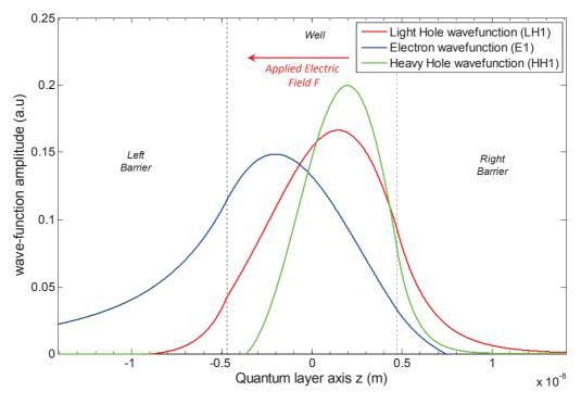
Figure A.3: Wave-functions for 1550 nm incident light under -3 V
