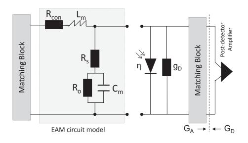
Figure 4.2: EAM quasi-static circuit model
