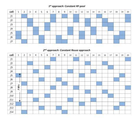
Figure 5.16: Illustration of both RF planning approaches for 20 cells network (2 RFs/cell).
