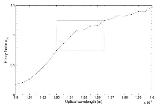
Figure A.7: EAM Henry factor  $(\alpha_H)$  as function of photon wavelength.
