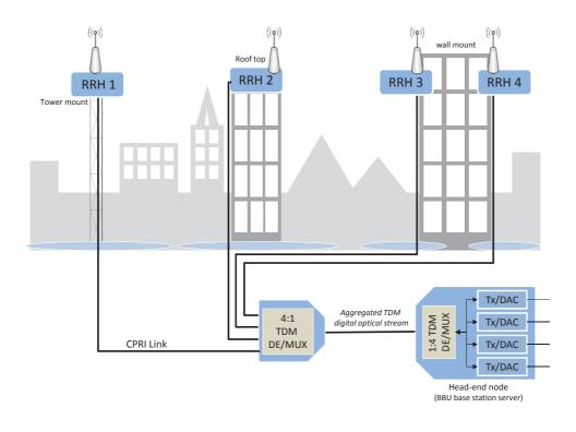
Figure 3.14: Distributed D-RoF architecture using CPRI.
