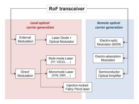
Figure 4.1: RoF transceiver technology classification.
