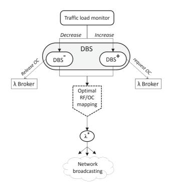
Figure 6.3: DBS activation by the GeRoFAN-CP and interaction with the  $\lambda$ -broker.
