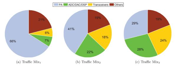
Figure 3.13: Power consumption profiling for 3 different traffic mixes.
