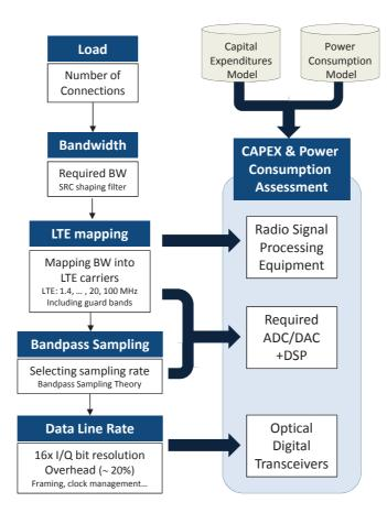
Figure 3.11: Methodology for A-RoF and D-RoF link modeling.
