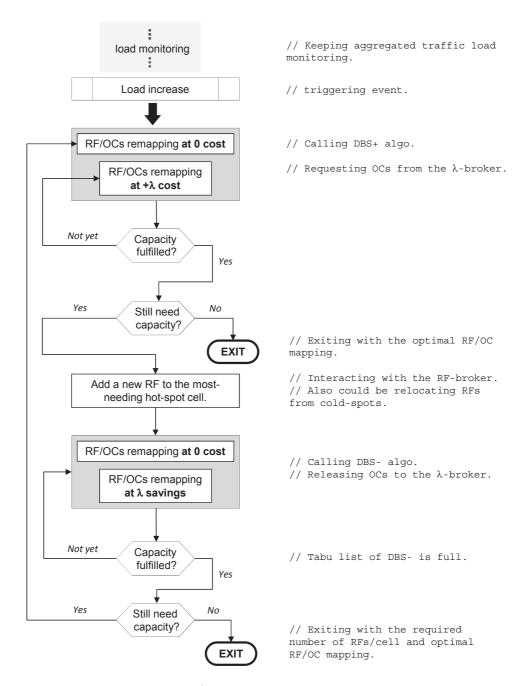
Figure 6.10: Flowchart of the radio/DBS cross-layer management approach for the case of a traffic increase.
