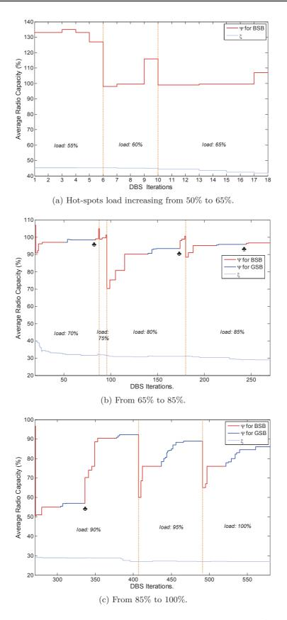
Figure 6.7: Running the DBS algorithm as the load in hot-spots increases.  $\clubsuit$  denotes the adding of a new OC. Attained *Incompressible Capacity*  $\simeq 27\%$ .
